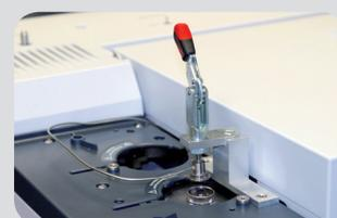
The UNIS **VOC Interface** is very suitable for volatile organic compounds, due to the septumless design. External sample systems, such as TDS or pyrolysis, can be connected fixed and gas tight via the integrated 1/16" connection.
