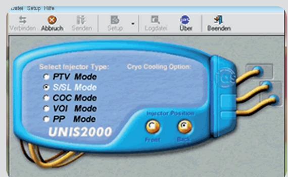
Changing from S/SL to PTV is done entirely through the software, without any changes to the inlet hardware. The total procedure takes only a few seconds. Switching to another mode, such as cool-on-column, is done by exchanging the injector body and entering the CoC parameters in the UNIS Configurator. After automatic GC reboot, the new injection mode is ready for operation.
