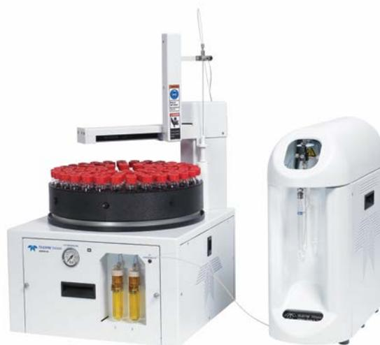
This study uses a Teledyne Tekmar Stratum Purge and Trap Concentrator (PTC) and AQUATek 100 Autosampler coupled to a Thermo ISQ Single Quadrupole GC-MS. A calibration curve and detection limits will be determined for the VOCs on the UCMR 3 analyte list.
