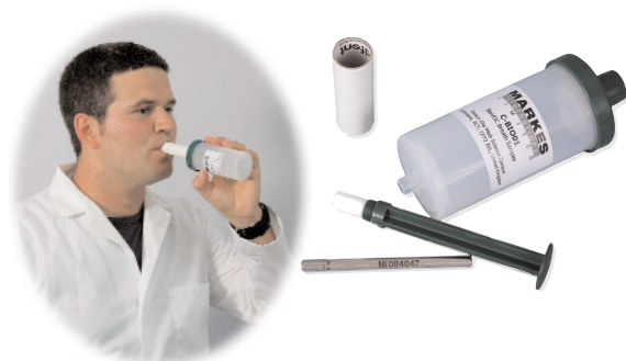
Figure 18: Bio-VOC™ Breath sampler (Markes International Ltd., UK) developed by UK HSL
