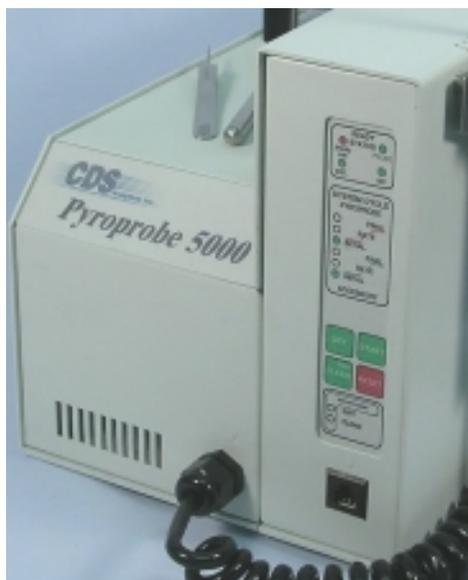
The front panel of the Model 5000 includes several LEDs for indicating the running status of the instrument plus keys which may be used to start and stop a method, run the dry function and run the clean function.
