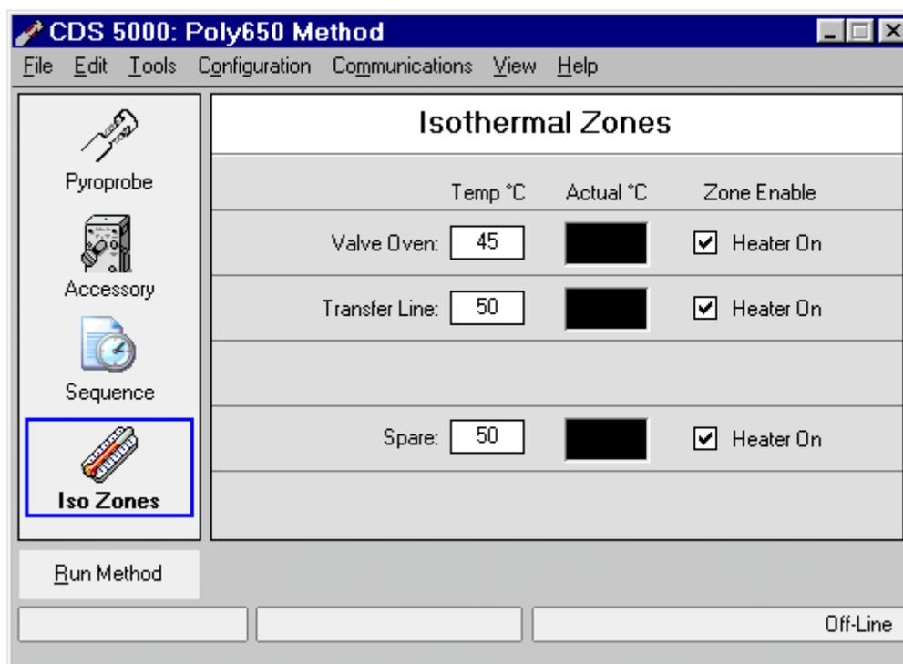
The Pyroprobe is capable of controlling up to four isothermal zones. For the 5150, two of these are pre-set as the valve oven (for the on-line/off-line valve) and the heated transfer line to the GC. These values are saved as part of the method. Each zone may be turned on or off by checking the *Heater On* box displayed in the *Iso Zones* screen.
