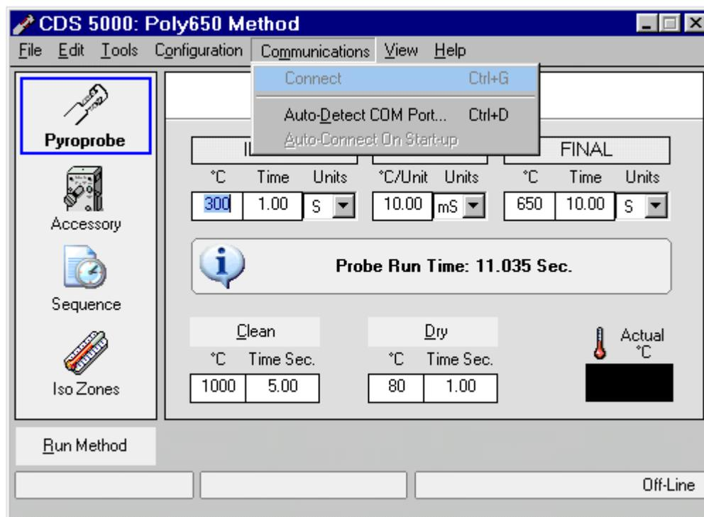
The *Communications* menu provides control of the communication between the PC and the 5000 unit itself. Clicking on the top entry (*Connect*) establishes communication to the 5000, which is confirmed by a tone at the 5000, at which time the top line changes from “Connect” to “Disconnect”.
