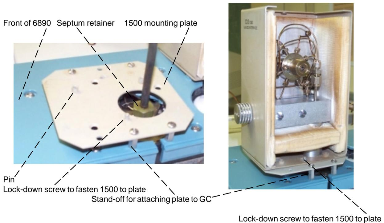
**FIGURE 5.4.** Mounting for Agilent 6890 GC.
