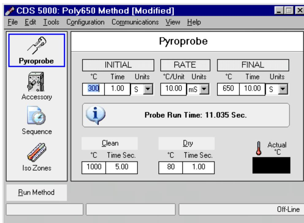
A method includes all parameters for the Pyroprobe filament, the interface zone, the clean and dry functions and the isothermal setpoints. The screens for setting parameters for each function are selected by choosing the appropriate icon on the left-hand side of the window. Selecting *Pyroprobe* presents the screen for entering the initial, rate and final setpoints for the filament itself, plus the clean and dry functions.
