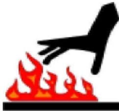
The Hot Surface Warning symbol is used to indicate the potential that the indicated surface may be hot and should not be handled until the unit has been turned off and the part has cooled.
