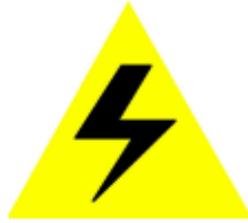
The Shock symbol is used on the Pyroprobe to indicate the potential for an electrical shock to the user, and that the Pyroprobe must be turned off and unplugged before accessing these parts.
