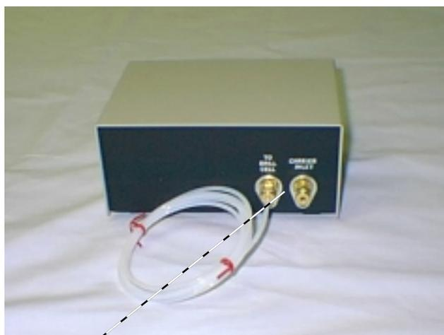
Bulkheads for flow in from tank and flow out to Brill Cell
