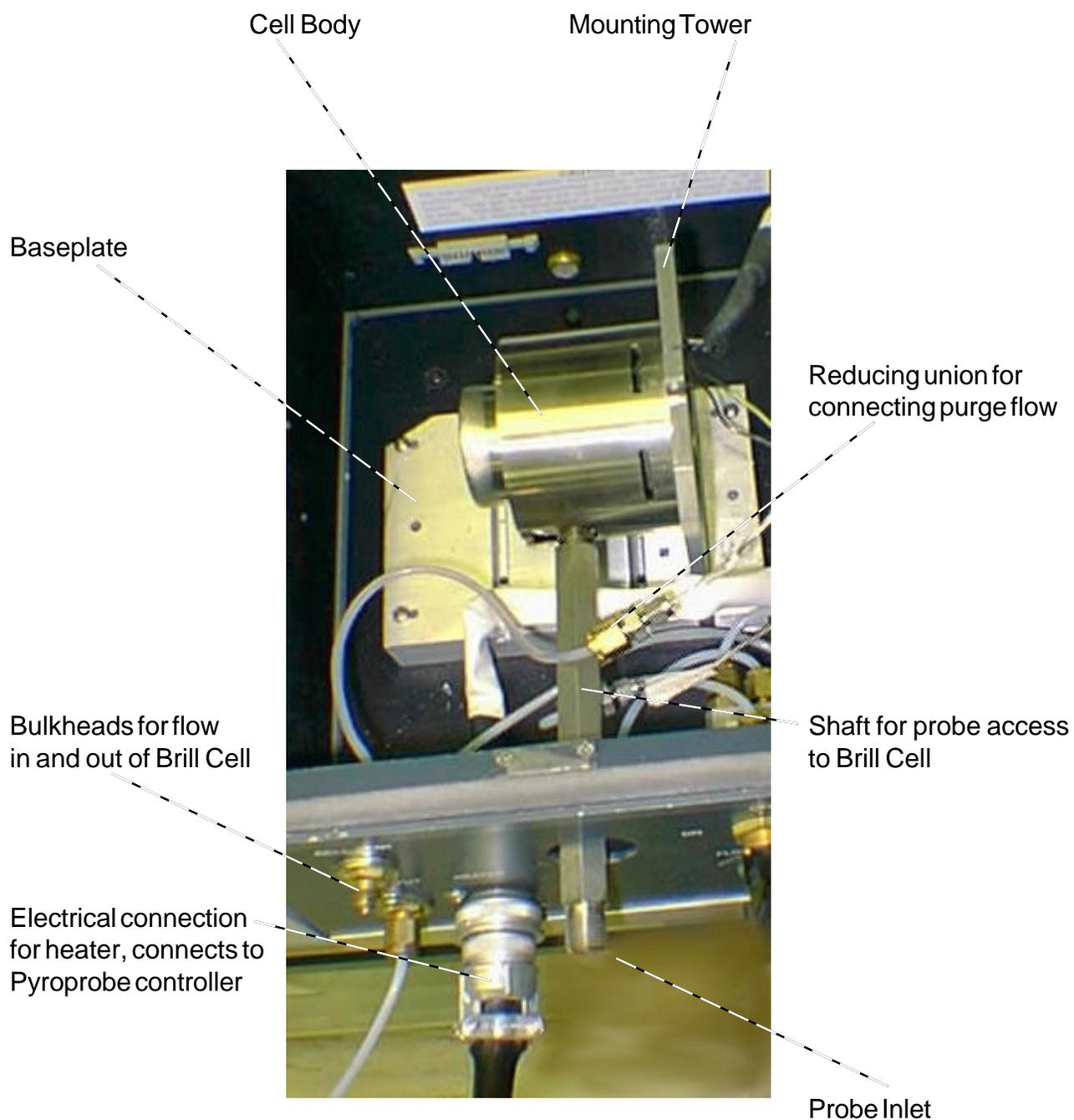
FIGURE 7.3. BRILL CELL AS SEEN FROM TOP IN INSTRUMENT.
