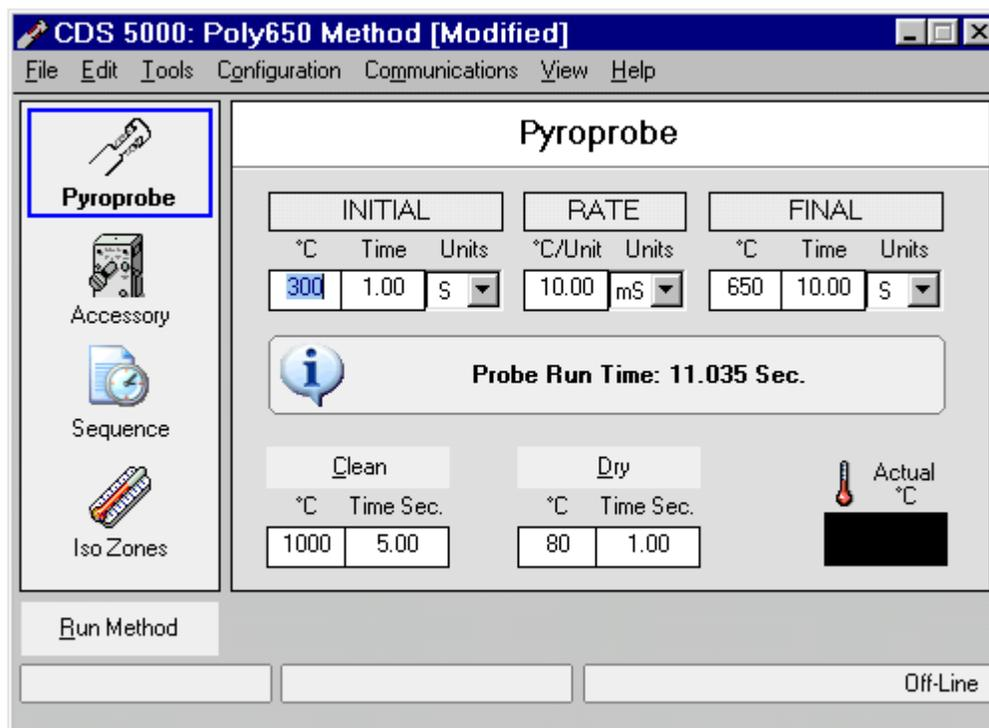
This base screen has icons on the left side for the Pyroprobe, the Accessory (interface) establishing a Sequence of methods and for displaying Isothermal Zones. Across the top of the screen is a menu bar with selections for:
