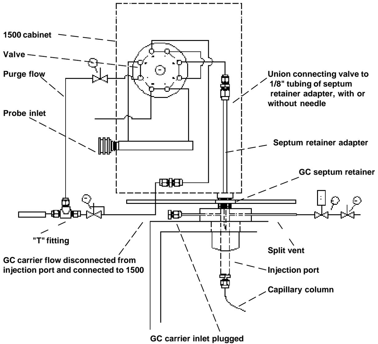
**FIGURE 5.2.** Pneumatic configuration.
