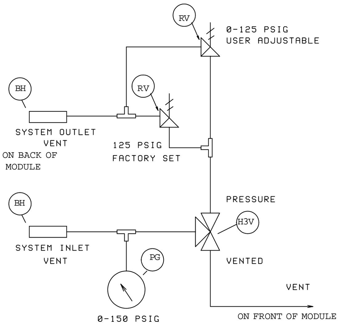
FIGURE 7.4 ELEVATED PRESSURE OPTION PNEUMATICS DIAGRAM.
