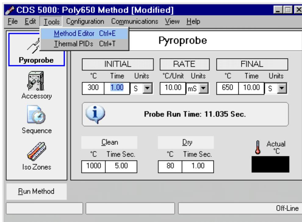
Selecting *TOOLS* from the menu bar provides two selections, the *Method Editor* and access to the *PIDs* for the various heaters. PID values are set for the heaters at the factory and under normal conditions require no adjustment by the user.
