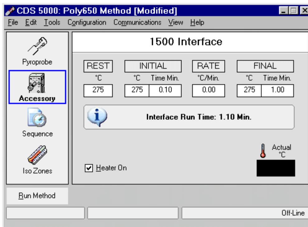
The interface zone for the Pyroprobe is also set in °C, with a maximum of 350°C. To prolong the life of the rotor used in the 1500 valved interface, a maximum extended use temperature of 300°C is recommended.
