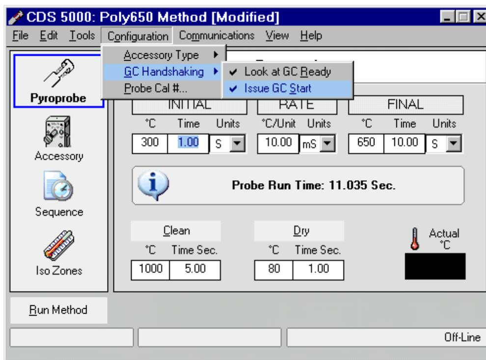
The *Configuration* menu includes selections for *Accessory Type*, *GC Handshaking* and is where the probe *Calibration* number is entered.
