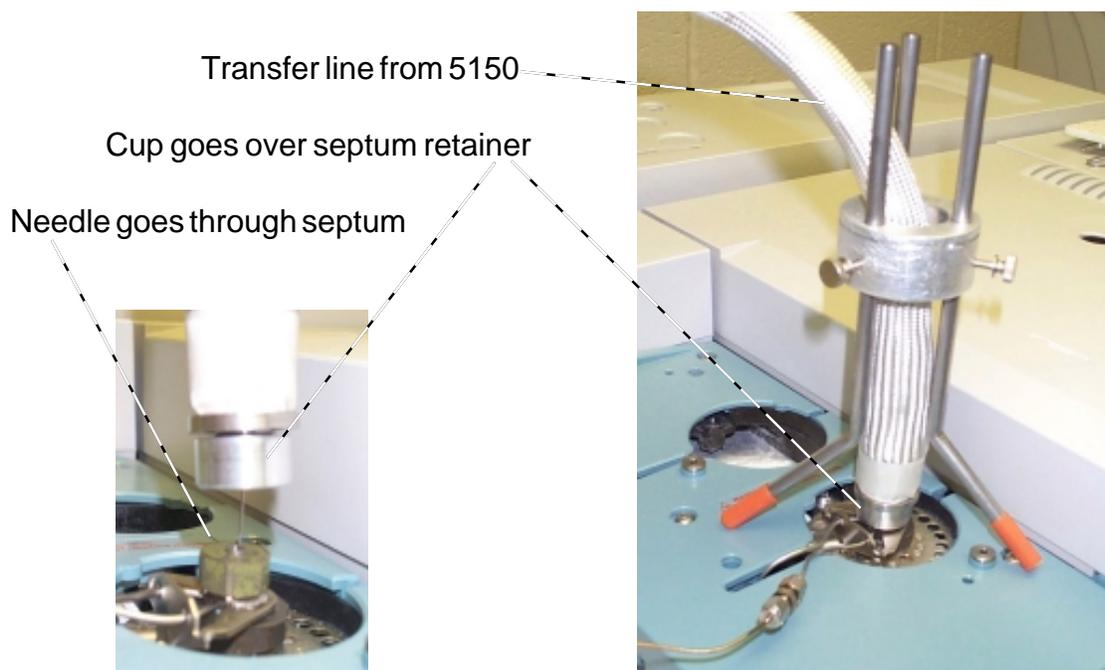
**FIGURE 5.8.** Heated transfer line at GC injection port.
