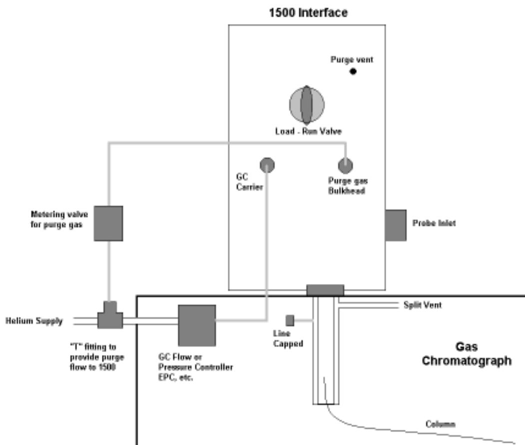
FIGURE 5.1. 1500 interface diagram.
