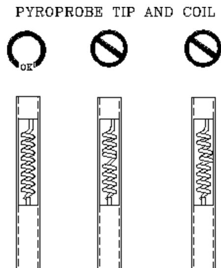
If the coil has become bent or distorted, it may be straightened using fine point tweezers. First, insert a quartz tube into the coil to stabilize it. Then using gentle pressure with the tweezers, adjust the loops of the coil so that they are not touching each other or the side of the probe.
