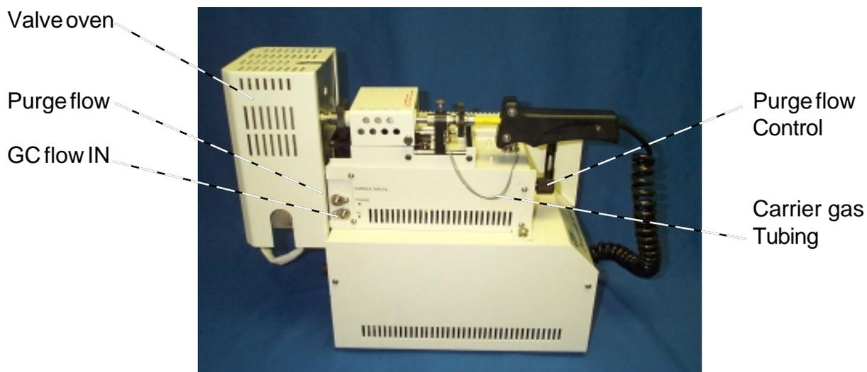
**FIGURE 5.7.** Pyroprobe 5150, side view.
