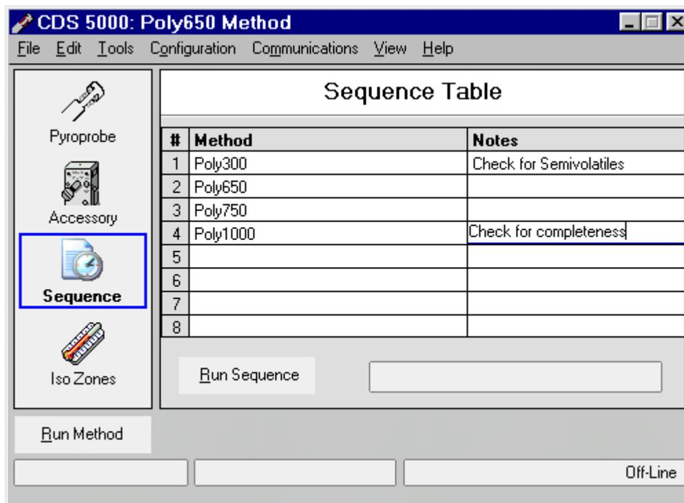
Once a sample has been loaded into the 5000 or 5150, it may be analyzed using several methods sequentially and automatically. Up to eight methods may be used in a sequence, each one with a pyrolysis and interface program, starting the GC each time. The use of the 5150 low-mass interface zone is especially useful in proceeding through a series of temperatures from low to desorb volatiles and semivolatiles to high for pyrolysis.
