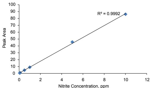
Fig. 2: Calibration Curve for Nitrite 0.05-10 ppm range
