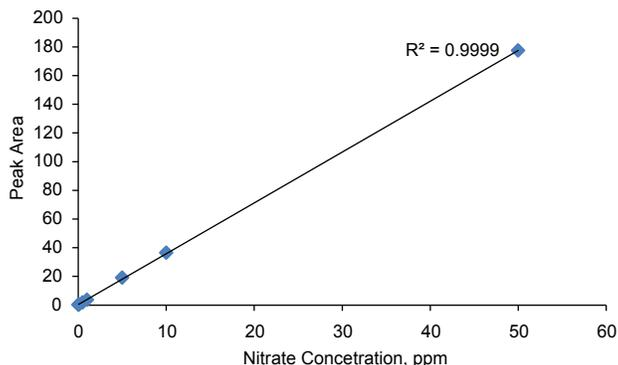
Fig. 1: Calibration Curve for Nitrate 0.05-50 ppm range
