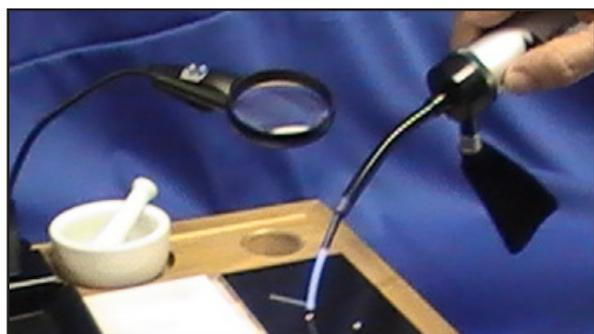
The compact vacuum pump allows you to easily draw solid samples into your quartz sampling tube.
