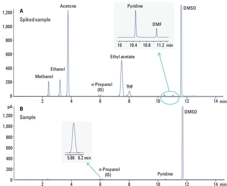
Figure 2. Chromatograms of standard spiked sample (A) and sample solution (B) using an Agilent HS/GC/FID system and an Agilent J&W DB-Select 624UI column.
