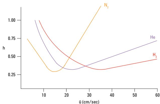
Figure 1. Van Deemter plot of helium, nitrogen, and hydrogen.
