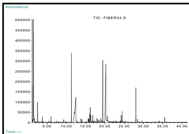
Figure 2. Pyrogram of PET pyrolyzed at 750°C.
