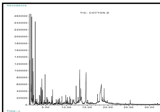
Figure 1. Pyrogram of cotton thread, pyrolyzed at 750°C.
