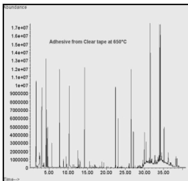
**FIGURE 4.** Pyrolysis of adhesive from clear tape.
