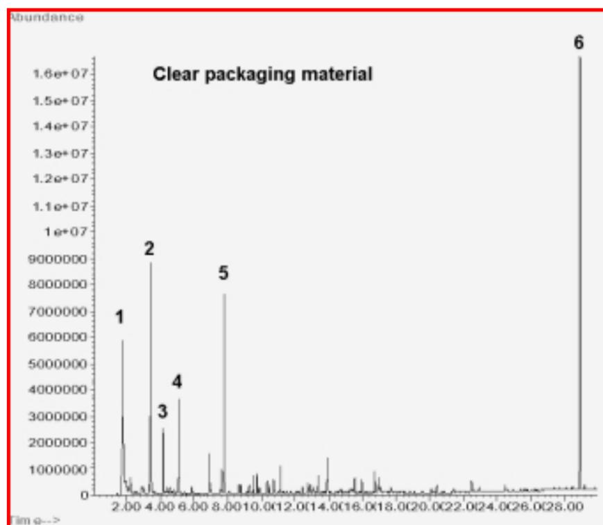
**FIGURE 1.** Pyrolysis at 700°C of a molded packaging product made from polystyrene, polymethyl methacrylate and polyvinyl chloride. The HCl, Benzene and Toluene are pyrolysis products of PVC.
