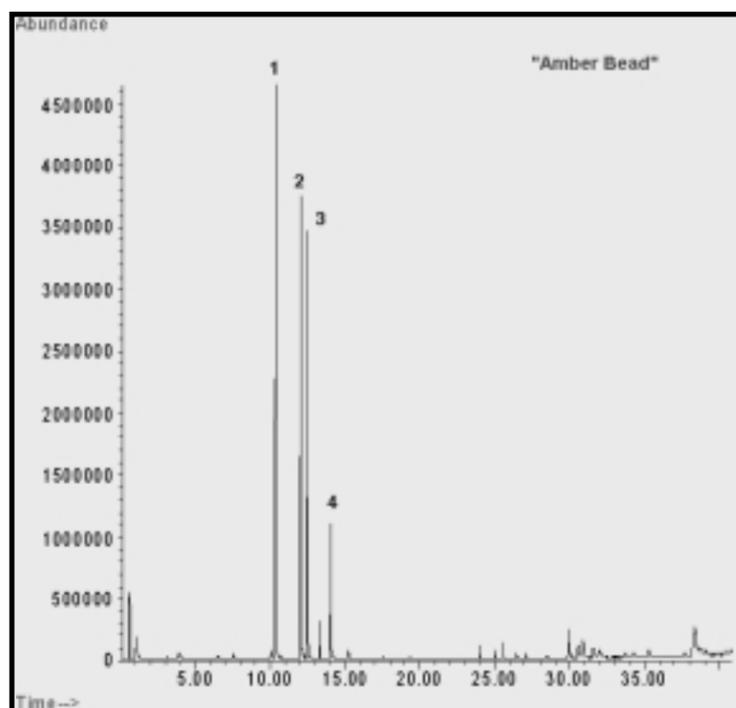
**FIGURE 2.** Pyrolysis of amber colored bead.
