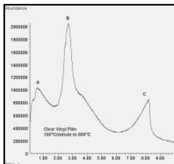
Figure 12. Clear vinyl film heated at 100°C/minute.
