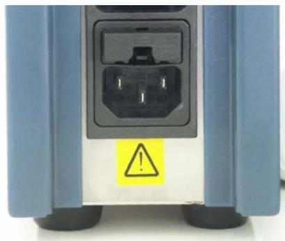
Connect the detector to a grounded AC power source, line voltage 100 – 240 VAC, frequency 50/60 Hz. The instrument should be connected to a protective earth via a ground socket. The power source should exhibit minimal power transients and fluctuations. Replace faulty or frayed power cords.
