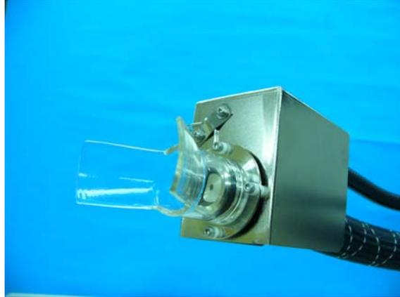
This is most suitable for identifying subtle scents and for highly skilled operators. The nose guard also prevents burns to the nose often caused by contact with metallic parts.
