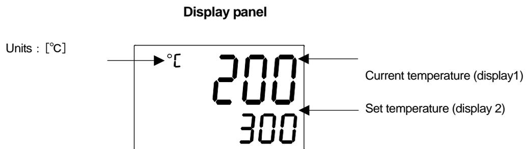
A screen similar to the one above appears when you turn the POWER switch ON. The current transfer line temperature appears in display 1 (red), and the set temperature appears in display 2 (green).
