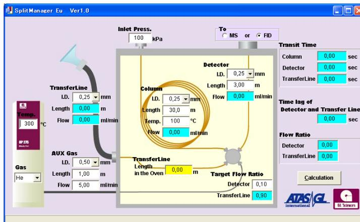
Conventionally, trial and error techniques are used to measure flow at each outlet to determine the optimum length and diameter for the capillary tube branching from the column. Split Manager provides a better solution than the troublesome procedure of having to repeatedly change columns and wait for the system to start up. Split Manager enables you to create a simulation beforehand and so setting up is quick and easy right from the beginning.
