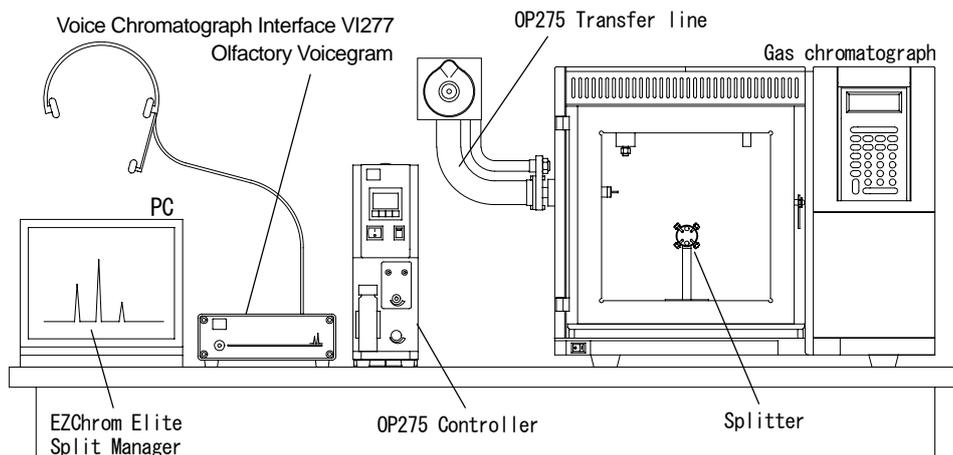
The OP275 is compatible with a wide range of gas chromatographs. And, since the transfer line does not have a cooling point, compounds with a high boiling point are less likely to leave residual odors around the outlet, removing the chance that subtle changes in scent may be missed, making it easier to determine compounds.
