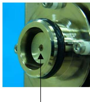
Set the tube flush with the heat block surface.
