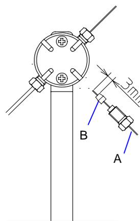
A : Fused silica capillary tube                    0.25 I.D.×0.35 O.D.
