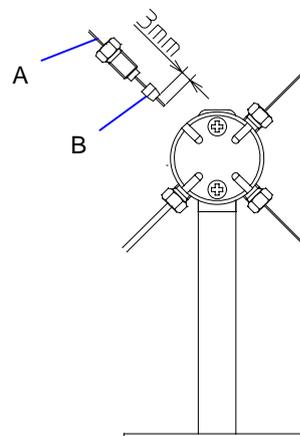
A : Fused silica capillary tube                      0.25 I.D.×0.35 O.D.
