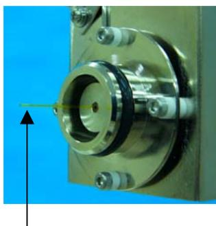
Push the tube in until it emerges from the heat block.
