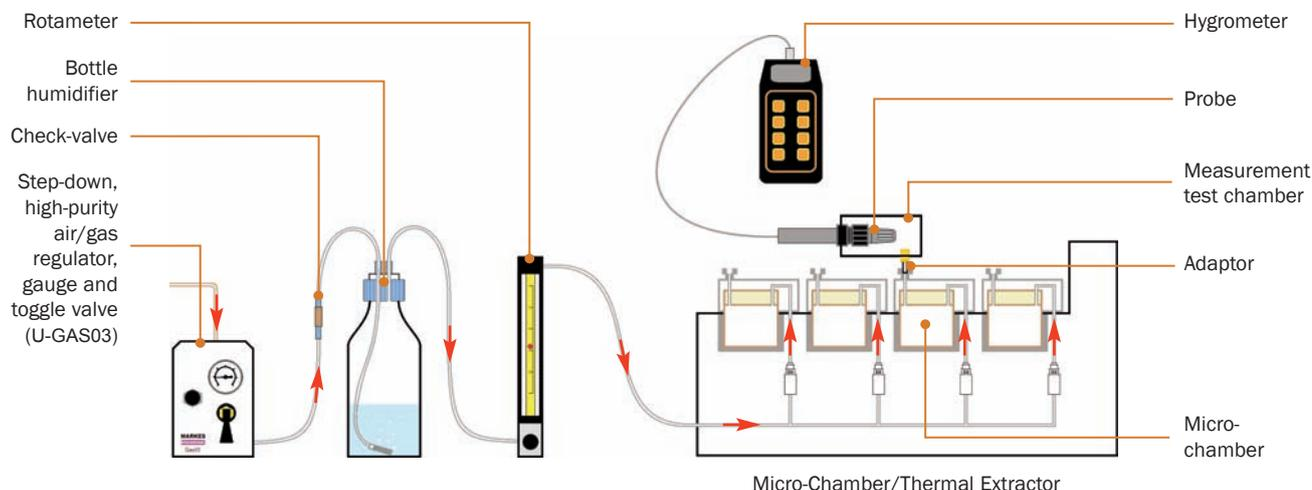
**Schematic of the Humidifier Accessory being used with a Micro-Chamber/Thermal Extractor**
