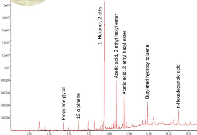
Surface emissions from a sample of vinyl flooring and adhesive tested using the  $\mu$ -CTE at 40°C with 50 mL/min air flow for 20 mins
