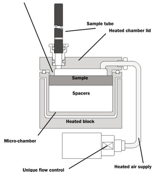
Schematic of single micro-chamber as used for surface emissions testing
