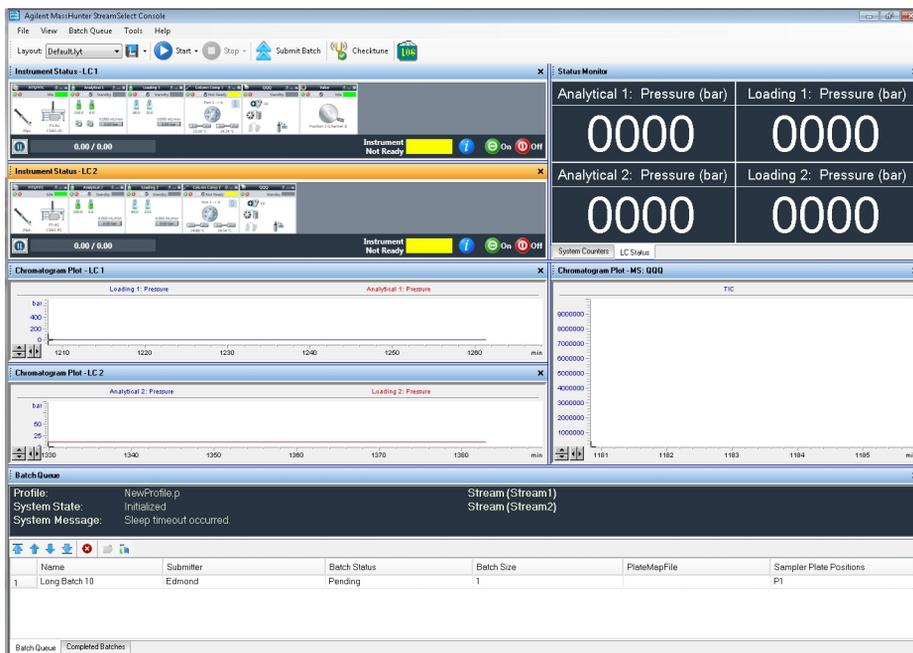
**Tip** The windows on the MassHunter StreamSelect Console can be resized, moved, or hidden to display only the information of interest. The layout can be saved; different layouts can be selected using the **Layout** controls on the toolbar.
