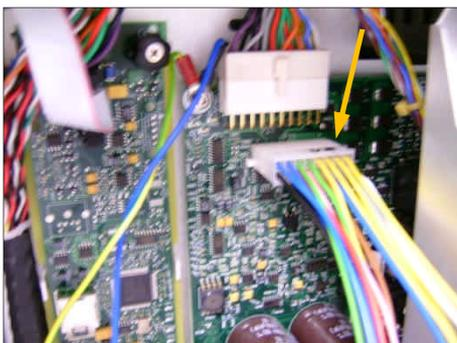
Fix the enclosed connector plug on the right board (see arrow).
