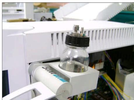
Put the water bottle for the sniffing gas humidification into the holder and connect the adapter of the frit with the humidification gas supply (e.g. humidifier out-port of the external pneumatic box, see 3.4). Put the flexible tube onto the second adapter. The other end is connected to the top of the transfer line (see next figure).
