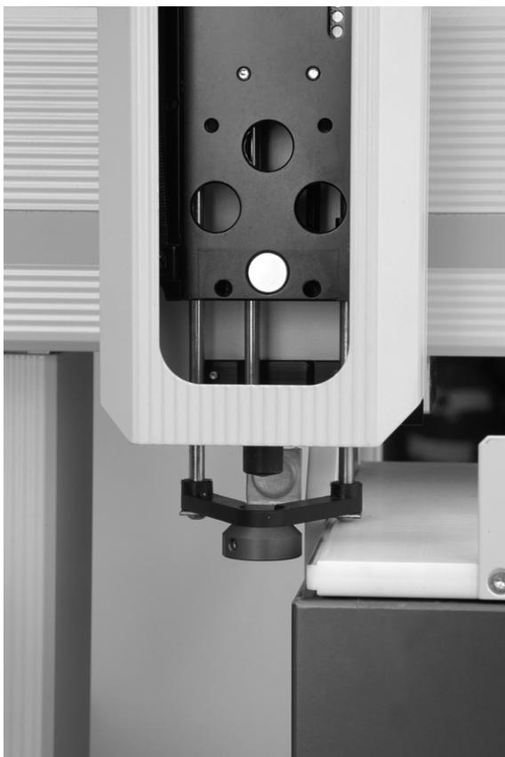
**Figure 4** Injection unit in the **FiberExp** position with the right edge just touching the left rear edge of the agitator
