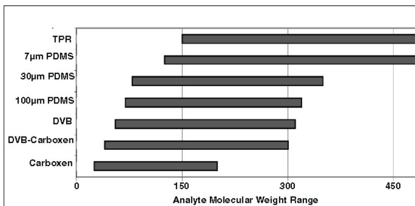
**Figure 3** Fiber coating type based on molecular weight range
