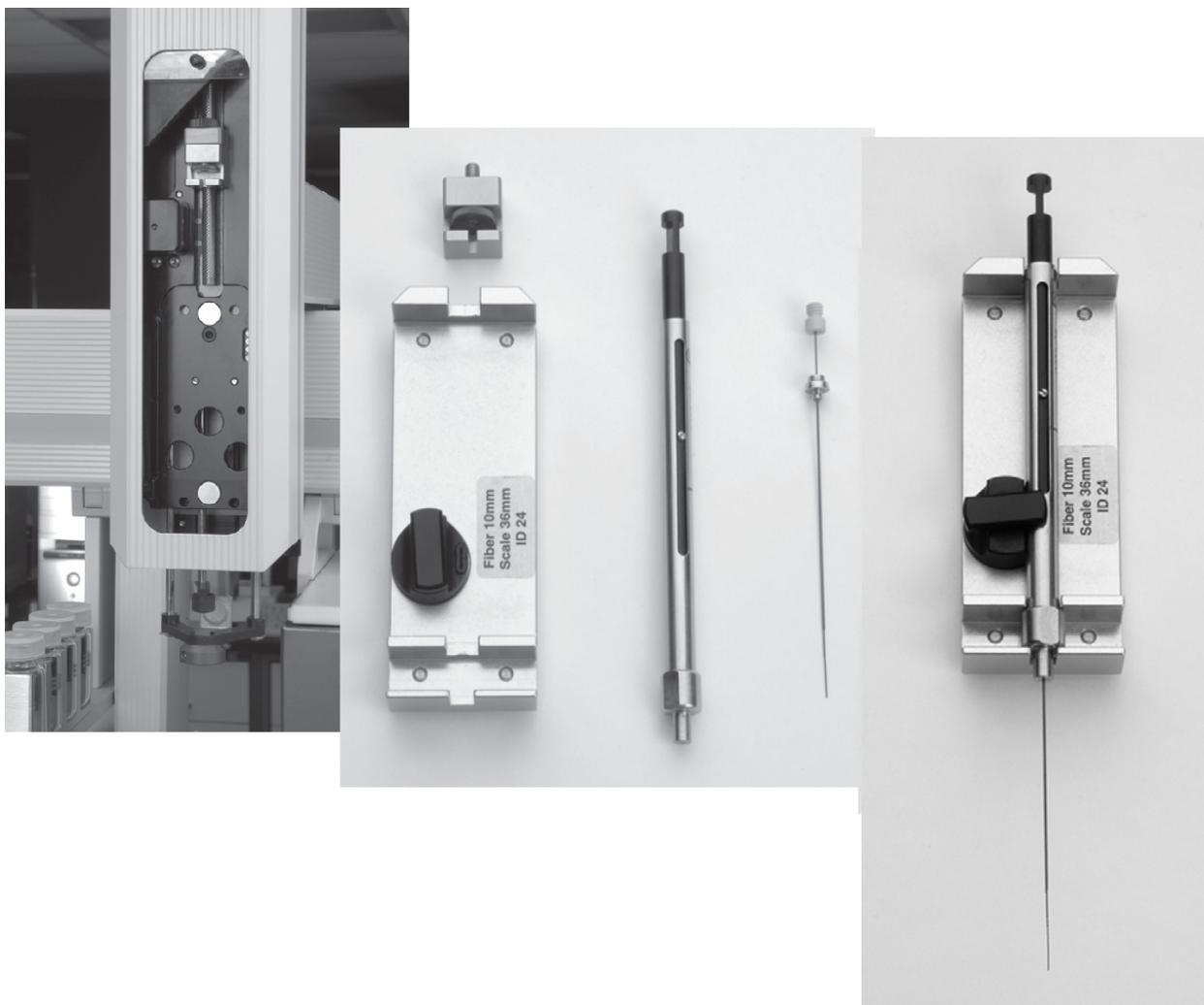
**Figure 5** Left: injector unit with plunger holder installed, Center: unassembled kit components; Right: fiber holder and fiber assembly properly installed in the PAL Autosampler SPME adapter
