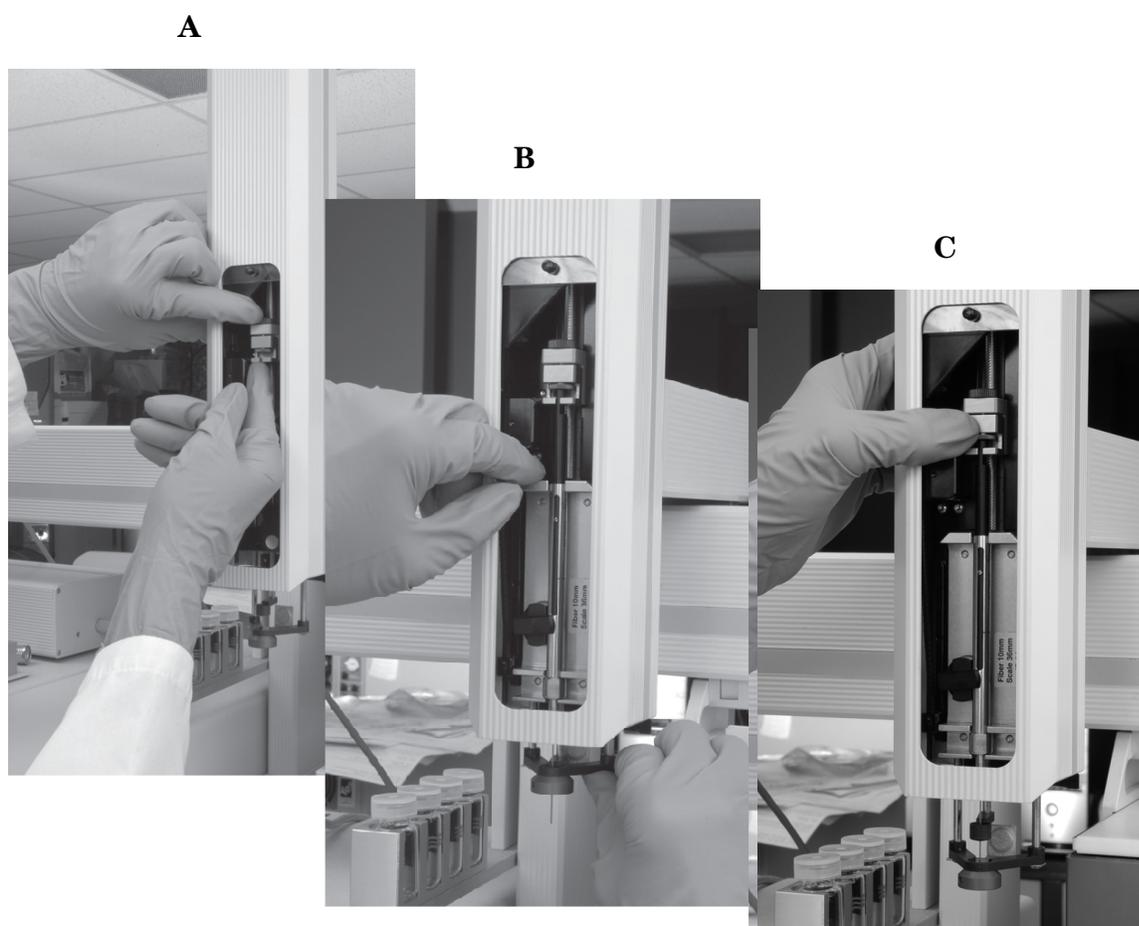
**Figure 6** Installing the fiber holder assembly
