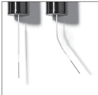
Needle bends during injection into sample vial or GC injection port
