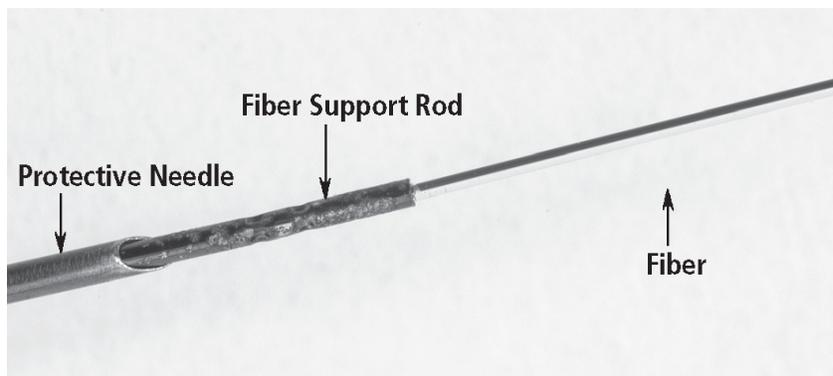
**Figure 1** Detail of the fiber assembly
