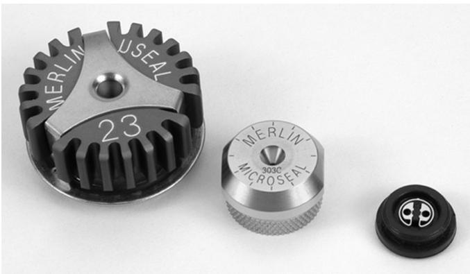
**Figure 2** The Merlin Microseal can be installed in a GC injector in place of a septum. The device contains a "duckbill" that allows a needle to enter the injector without leaking.
