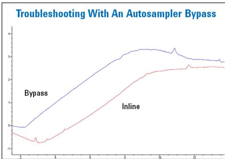
Extra peaks in the chromatogram, particularly with gradient analysis, may also be coming from the mobile phase. In the most extreme of examples of troubleshooting, we have bypassed the autosampler by connecting the pump directly to the column and running a blank gradient.
