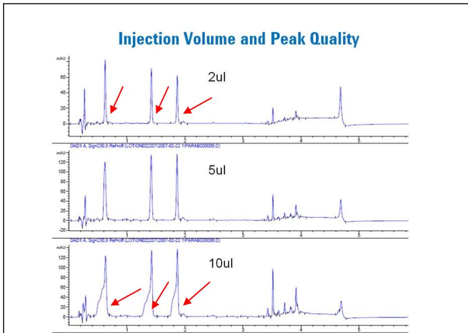
Injection volume will affect peak width, as we discuss in the Peak Broadening segment of the LC Troubleshooting Video Series. The example to the left shows injections at 2  $\mu$ l, 5  $\mu$ l and 10  $\mu$ l to demonstrate this concept. Note the various differences in peak width on peaks 2-4.
