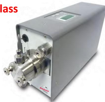
The compact M1 Class consists of single-headed, positive displacement piston pumps that deliver high-performance and precision at an affordable price. Applications include precise chemical metering, dispensing, and specific HPLC separation. Having the smallest possible footprint for a high pressure pump, the M1 Class will easily integrate into any laboratory or industrial environment.
