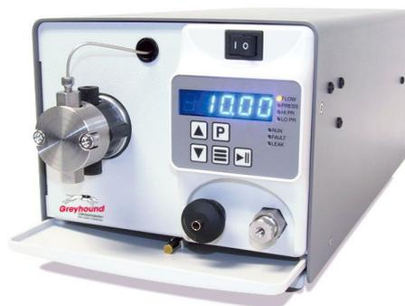
The reliable LS/LST Class consists of single-headed positive displacement piston pumps incorporating advanced cam designs for very low pulsation. With micro-stepping motor technology and a proven single-piston pump mechanism, the LS/LST Class exceeds the performance of more expensive units at a fraction of the cost. The pumps are ideal for a wide variety of HPLC applications (including biocompatible separations), semi-prep LC, metering & dispensing, and general lab use.
