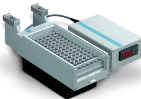
*The Peltier-cooled trayholder is ideal for thermally labile samples.*
