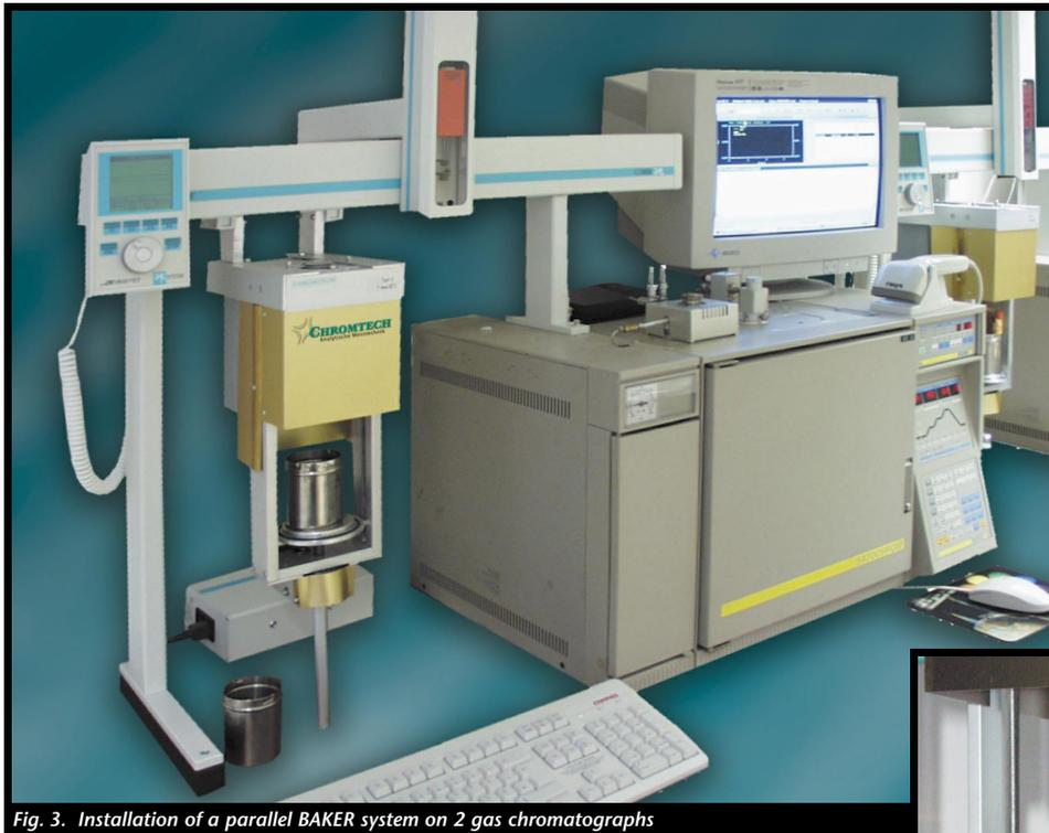
Fig. 3. Installation of a parallel BAKER system on 2 gas chromatographs
