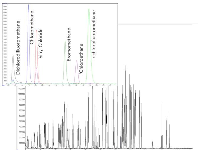
The Eclipse was used to prepare a chromatogram of an expanded list of USEPA Method 8260 standard. It illustrates superb chromatographic performance with baseline resolution for all light gases and polar compounds, even with high-speed columns.
