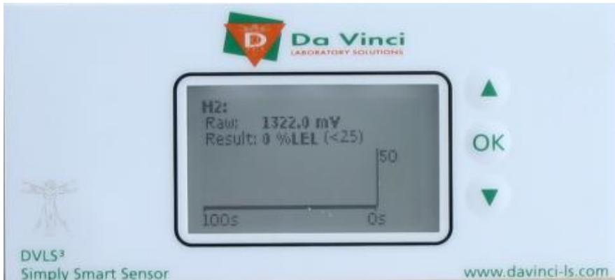
The Raw data figure corresponds to the actual signal from the sensor. The Result value is a relative measure of the actual Hydrogen level. Between parentheses the default alarm level is shown.
