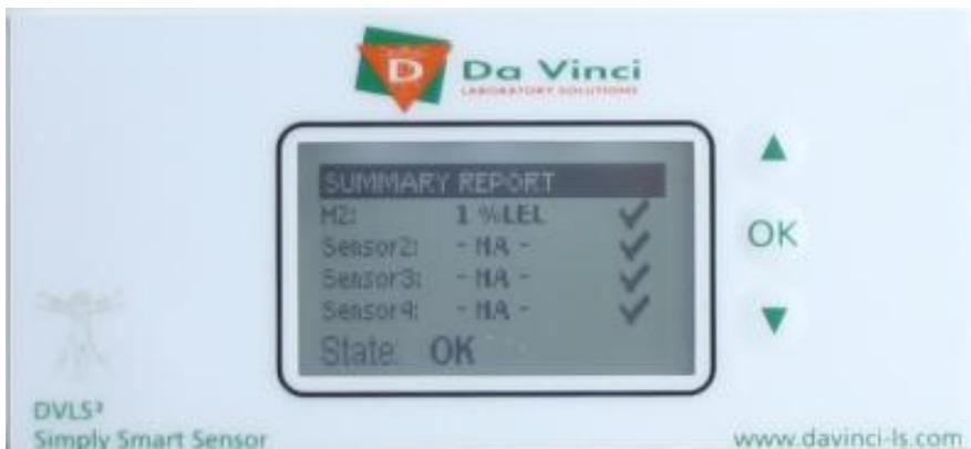
Submenus are accessed by using the arrows next to the display. When an individual sensor is accessed, the following screen becomes available:
