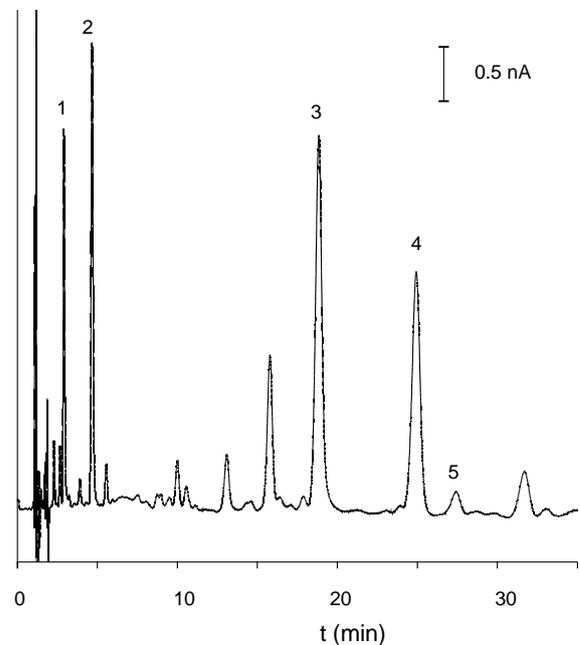
Fig. 1. Analysis of VMA, HVA and 5-HIAA in human urine. Peaks are: 1: VMA (26.7 µmol/l), 2: iso-VMA (IS), 3: 5-HIAA (66.4 µmol/l), 4: 5-HICA (5-hydroxyindolecarboxylic acid, IS), and 5: HVA (66.4 µmol/l). Courtesy: Dhr. J. van der Kolk, Clin. Chem. Lab., Bethesda Hosp., Hoogeveen, The Netherlands.
