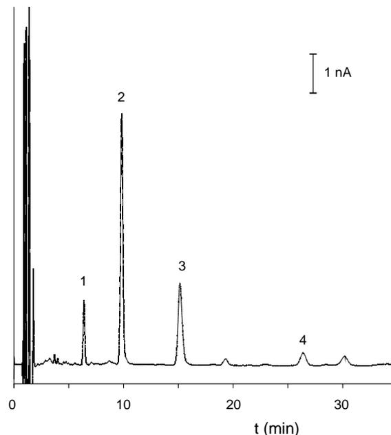
Fig. 1. Analysis of human urine. Peaks are: 1: normetanephrine (0.9  $\mu\text{mol/l}$ ), 2: metanephrine (8.2  $\mu\text{mol/l}$ ), 3: hydroxymethylbenzylamine (IS), and 4: 3-methoxytyramine (0.5  $\mu\text{mol/l}$ ). Courtesy: Dhr. J. van der Kolk, Clin. Chem. Lab., Bethesda Hosp., Dr. G.H. Amshoftweg 1, 7909 AA Hoogeveen, The Netherlands.
