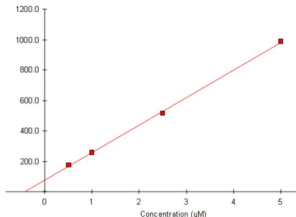
Fig. 1. Regression line of standard addition analysis of iodide in diluted and filtrated urine (see results in Fig. 2).
