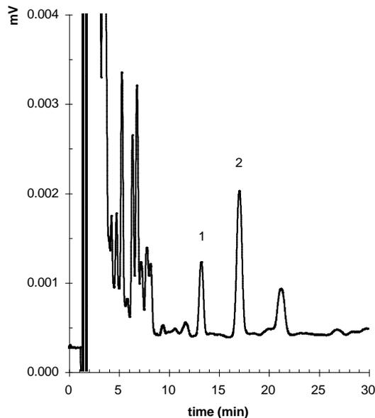
Fig. 1. Chromatogram of 5-HT (1) and nMet (2, IS) in human plasma. Concentration is 1 ng/ml. Courtesy: J.C.M. Schouten - Verhagen et al., Rijneest Group, Oegstgeest.
