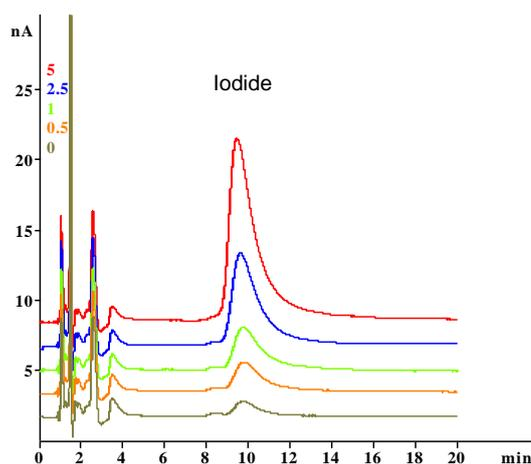
Fig. 2. Standard addition analysis of iodide in diluted (factor 10) and filtrated urine using ECD with a silver working electrode (20  $\mu\text{L}$ ). From top to bottom: urine with addition of 5, 2.5, 1, 0.5 and 0  $\mu\text{mol/L}$  potassium iodide. Peak height of iodide (at  $t = 10$  min) corresponds to a concentration of 4  $\mu\text{mol/l}$  in urine.
