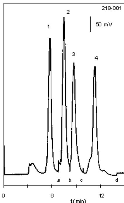
Fig. 1. Analysis of human LDL. Concentrations (amounts) are: 1. *a*-tocopherol (vitamin E) 3.6  $\mu$ mol/l (72.9 pmol), 2. ubiquinol-9 0.77  $\mu$ mol/l (15.5 pmol), 3. ubiquinol-10 0.21  $\mu$ mol/l (4.2 pmol), and 4. *b*-carotene 0.11  $\mu$ mol/l (2.2 pmol). The range is programmed at 10 (t=0), 1 (a), 0.5 (b), 1 (c) and 10 nA/V (d). Courtesy ref [1].
