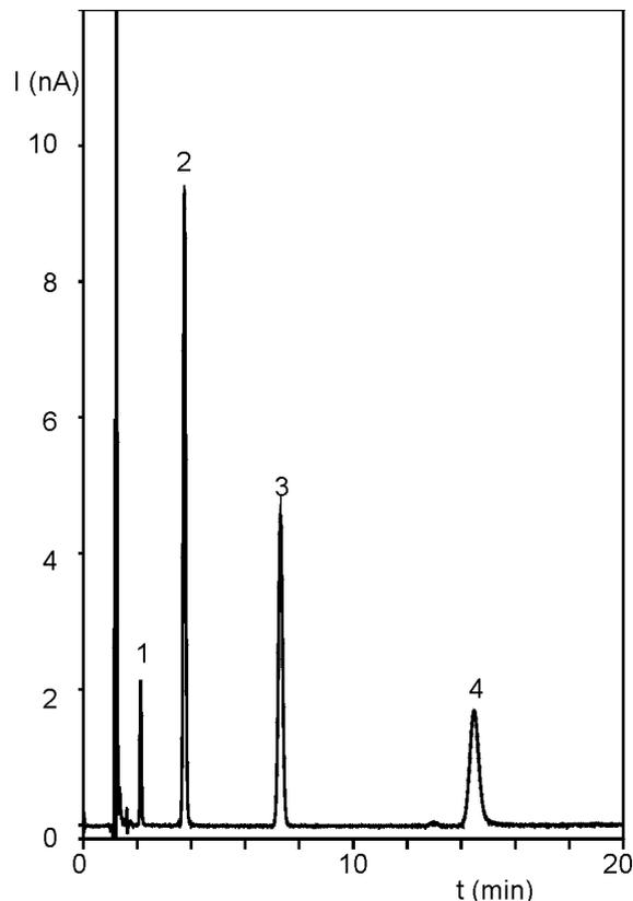
Fig. 1 Chromatogram of ascorbic acid (1) in pretreated plasma. Plasma concentration is 41  $\mu\text{mol/l}$ . Other peaks are: Urate (2), Hydrochinon (IS, 3) and DTT (4). Courtesy: M. van der Horst, M.G.J. Lunenburg and E. Oeben, Scheper Ziekenhuis, Emmen, The Netherlands.
