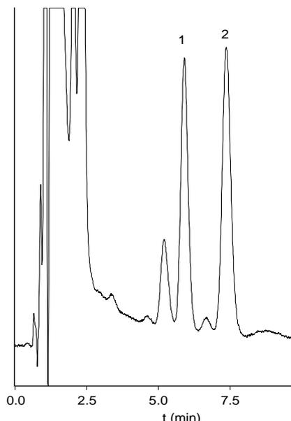
Fig. 2 Analysis of vitamin K1 (1) in plasma extract. Concentrations are 2.5 ng/ml for vitamin K1 and 5 ng/ml for internal standard 2,3 hydrophyllquinon.
