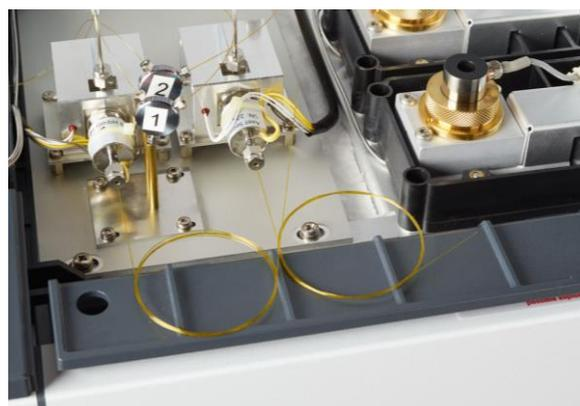
Figure 1: Heated valve unit.
