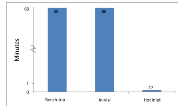
Figure 6. Time required to perform derivatization with bench-top methods, automated, in-vial methods, and hot inlet methods.
