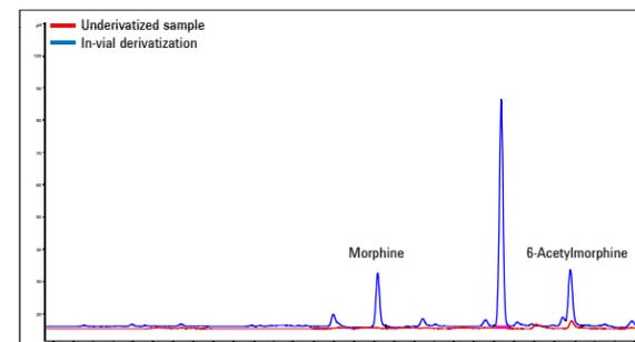
Figure 5. Chromatograms of morphine and 6-acetylmorphine underivatized and derivatized with 1 µL of BSTFA per µL of sample in the hot inlet.
