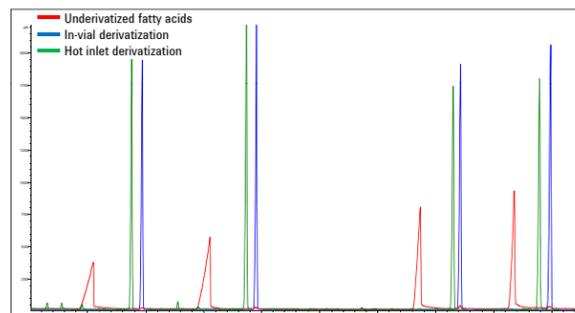
Figure 3. Chromatograms of fatty acids before derivatization, after in vial derivatization, and after hot inlet derivatization. The hot inlet derivatization chromatogram (green) is offset slightly for clarification.
