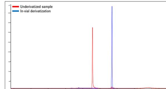
Figure 4. Chromatograms of pentachlorophenol before derivatization and after hot inlet derivatization. Prior to derivatization, the area RSD was 4.2%. After derivatization with BSTFA, the area RSD decreased to 1%
