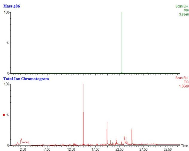
Figure 1. TIC (bottom) and mass 486 (top) for desorption of polymer.
