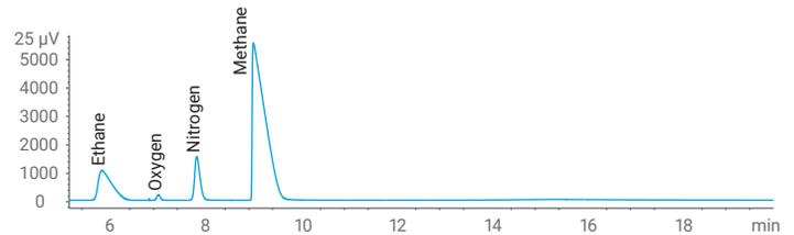
Methane, ethane, and permanent gases (oxygen, nitrogen, carbon dioxide) measured using a TCD channel with packed column.
