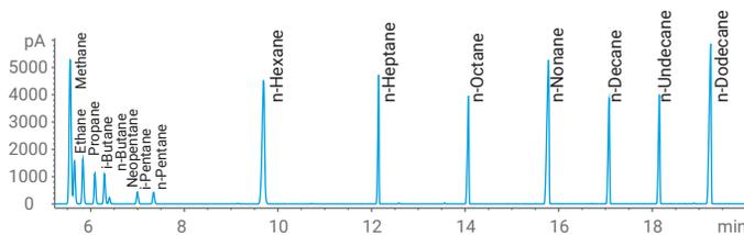
Hydrocarbons (C<sub>3</sub>-C<sub>12</sub>) separated on a PONA column and measured on FID.
