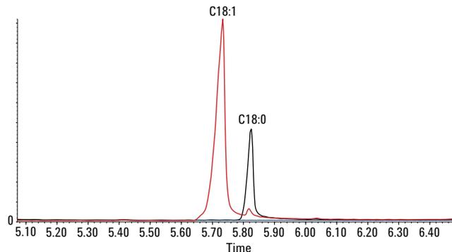
Figure 4. Separation of critical pair oleic (C18:1) from stearic (C18:0) acid.
