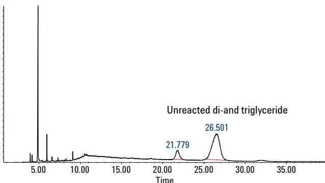
Figure 3. Agilent 7696A Prep WorkBench reaction at approximately 50% completion using GC conditions to elute all reactants.
