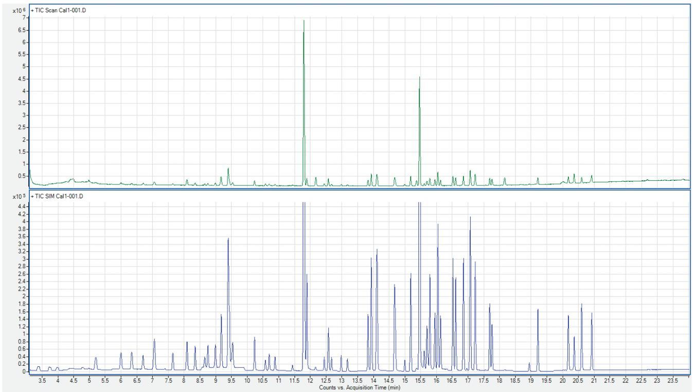
**Figure 2: 1 µg/L VOC Standard Scan and SIM Traces.**
