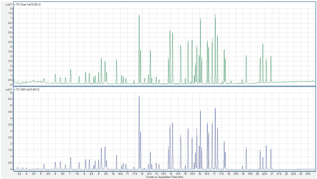
**Figure 1: 10 µg/L VOC Standard Scan and SIM Traces.**
