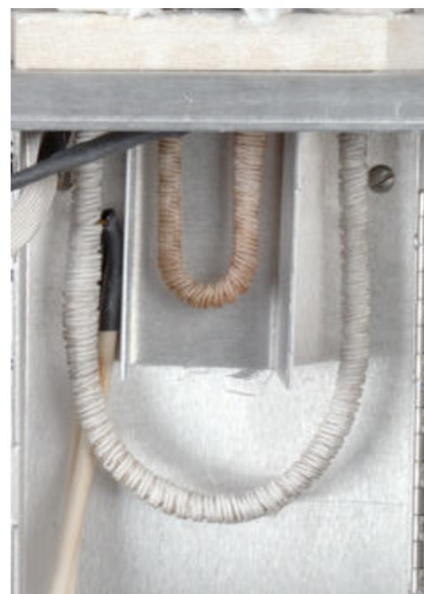
Stratum PTC Newly Designed U-shaped Analytical and Condensate Traps
