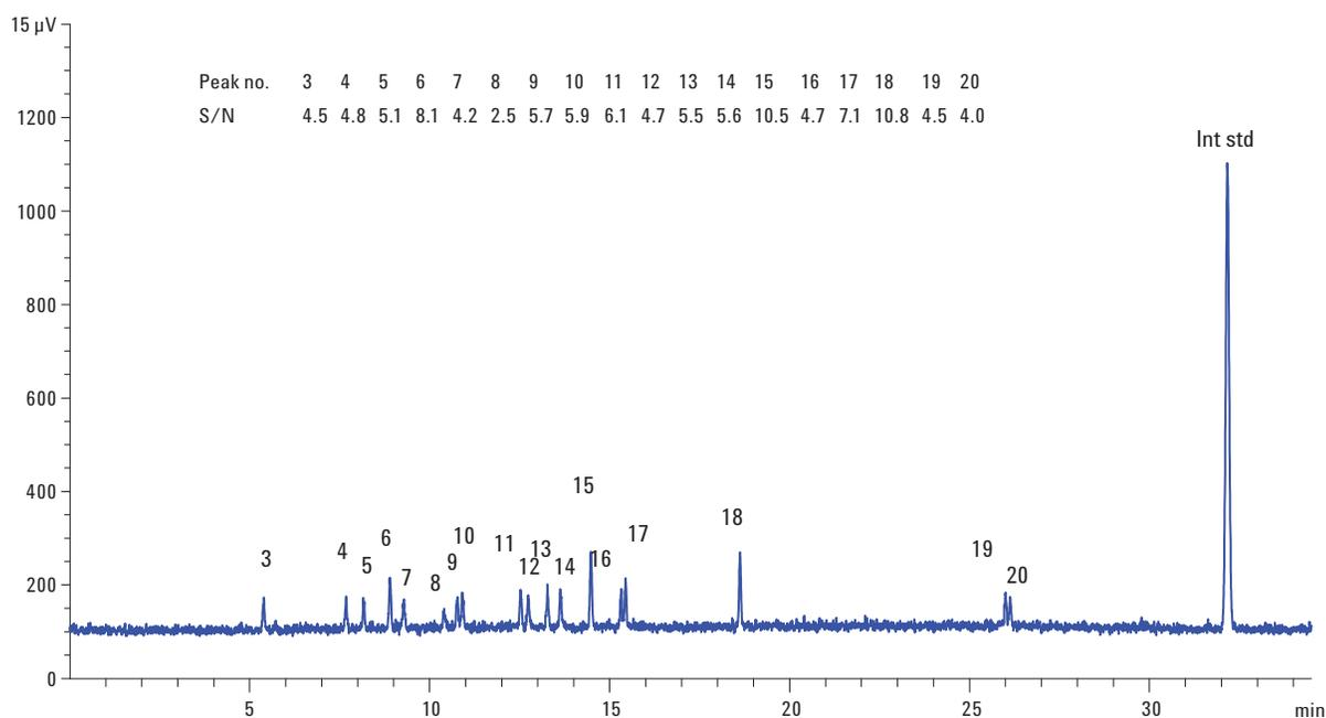
Figure 2. Chromatogram and signal-to-noise of sulfur standards at 0.1 mg/kg (approximately 0.01 ng on column). Refer to Table 1 for peak identification.
