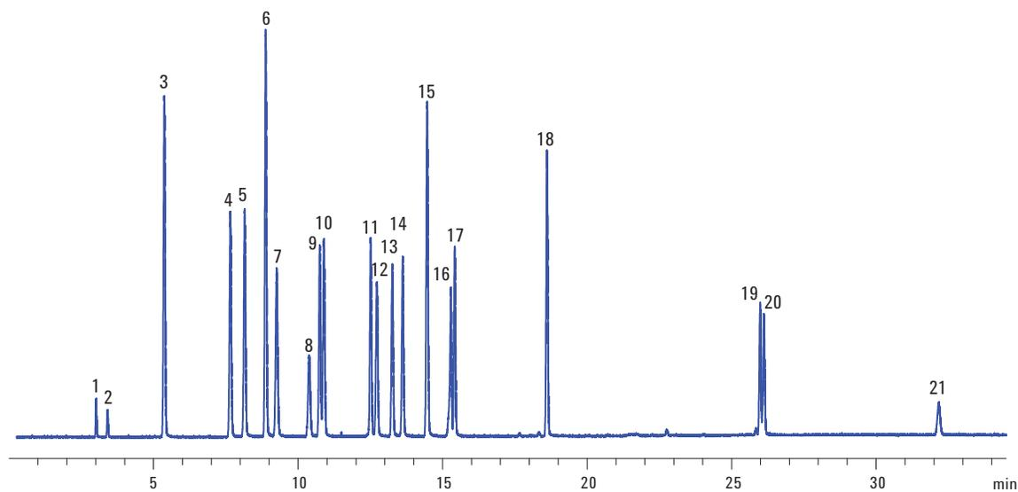
Figure 1. Chromatogram of sulfur standards in toluene using an Agilent GC/SCD system and Agilent J&W DB-Sulfur SCD column. Refer to Table 1 for peak identification.
