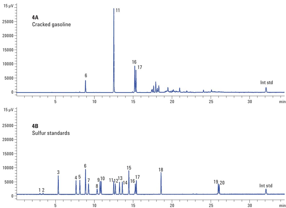
Figure 4. The chromatogram of a cracked gasoline sample that included more than about 63.5% aromatic hydrocarbons and 25% nonaromatic hydrocarbons (above). Chromatogram of sulfur standards at 5 ppm (below).
