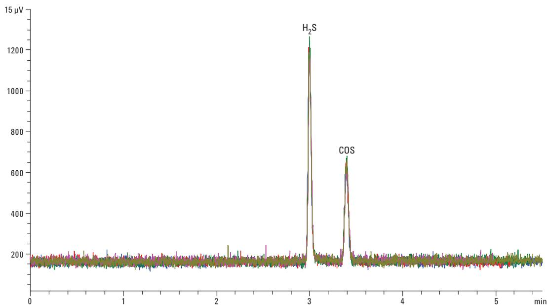
Figure 3. Chromatogram overlay of hydrogen sulfide and carbonyl sulfide at 2 ppm
