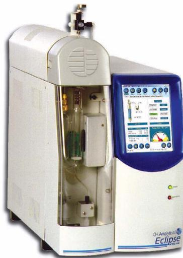
Figure 1. OI Analytical Model 4660 Eclipse Sample Concentrator
