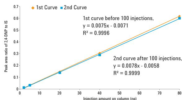
With improved deactivation, Ultra Inert liners – even with wool – provide excellent linearity over an extensive calibration range (2 to 80 ng) for active compounds like 2,4-Dinitrophenol.
