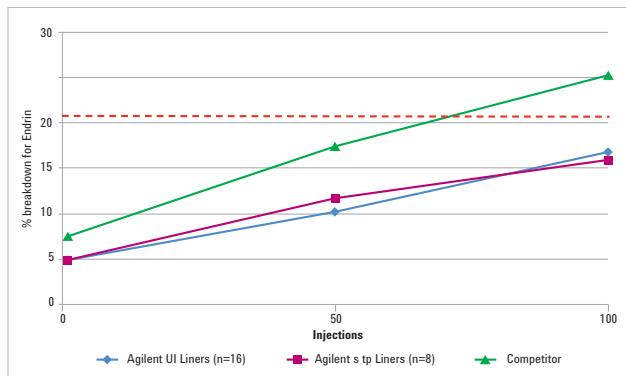
Agilent Ultra Inert Liners with wool are superior vs. the competition as shown in this Endrin breakdown comparison.
