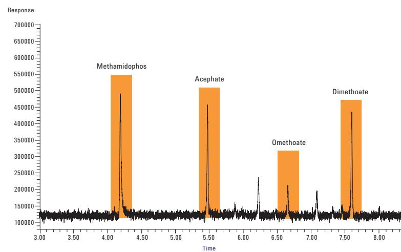
GC/FPD chromatogram (enlarged section) of a 15 ng/mL matrix-matched pesticide standard with analyte protectant, analyzed on an Agilent J&W DB-35ms Ultra Inert capillary column.
