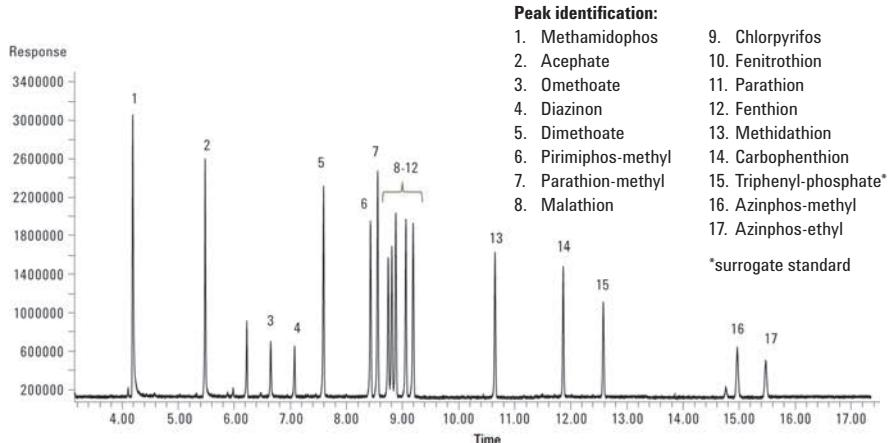
GC/FPD chromatogram of a 100 ng/mL matrix-matched organophosphorus pesticide standard with analyte protectant analyzed on an Agilent J&W DB-35ms Ultra Inert 30 m x 0.25 mm, 0.25 µm capillary GC column (Agilent Part No. 122-3832UI).
