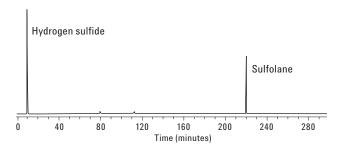
This particular LPG sample passed the copper strip corrosion test and yet contained over 40 ppm hydrogen sulfide by weight, according to stain tubes. Presence of polar compounds masked the corrosion effect of hydrogen sulfide. Their presence resulted from a unit upset in which gas treating chemicals were "burped" into a finished LPG storage jug. Presence of sulfolane also indicated the presence of amine treating compounds, since they are used simultaneously for sulfur compound removal.
