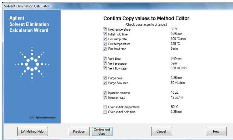
**Figure 5** Inlet and injection parameters determined by the Solvent Elimination Calculator for a 10-µL injection of a sample in acetonitrile with the approximate boiling point of the first analyte set to 150 °C
