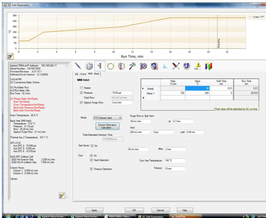
**Figure 1** Multimode Inlet setup screen for the PTV Solvent Vent mode
