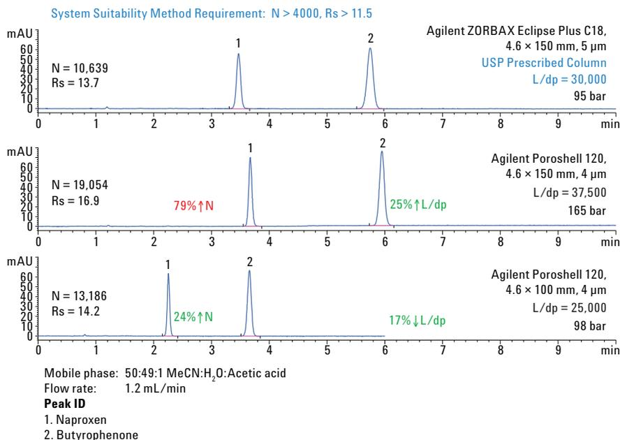
Figure 2. USP analysis of naproxen using Agilent Poroshell 120, 4 µm and Agilent ZORBAX Eclipse Plus, 5 µm columns. The 4 µm particles deliver a 79% increase in efficiency at roughly the same run time in the 150 mm column, or a 24% increase in efficiency with a 33% shorter run time in the 100 mm column.
