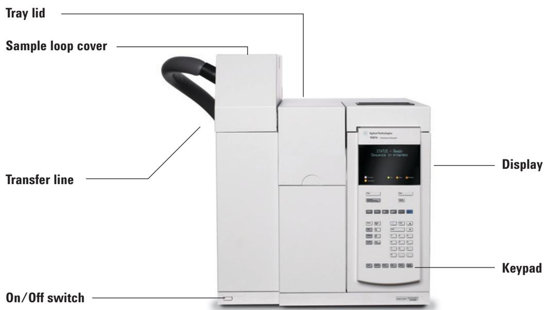
**Figure 2** 12 Vial model—front view
