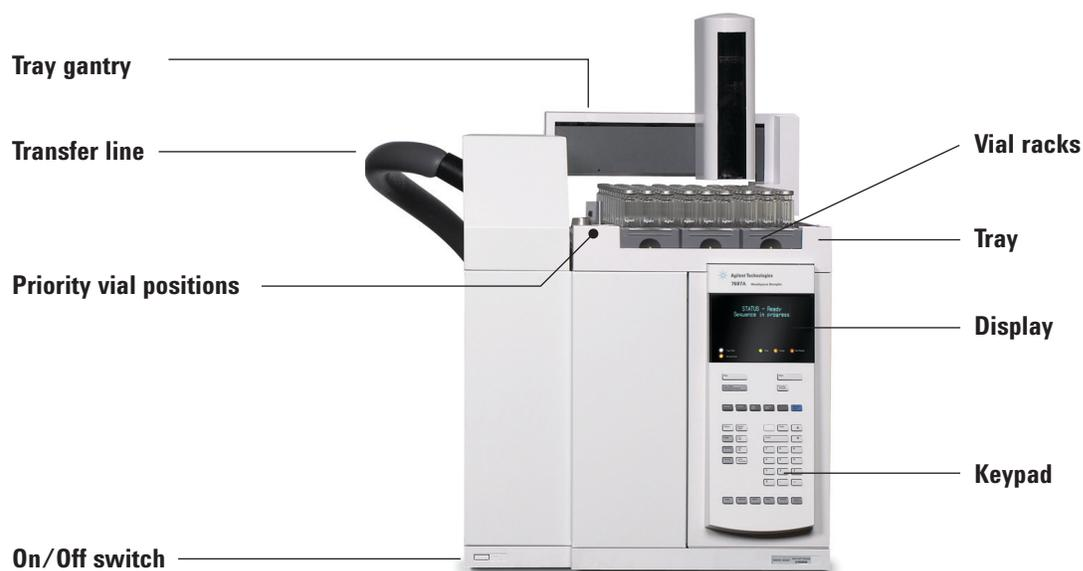
**Figure 1** 111 Vial model—front view
