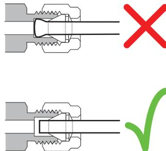
**Figure 30** Completed fitting
