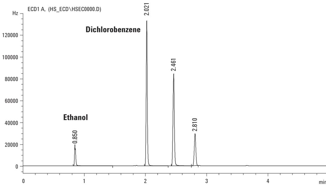
Figure 23 µECD checkout chromatogram
