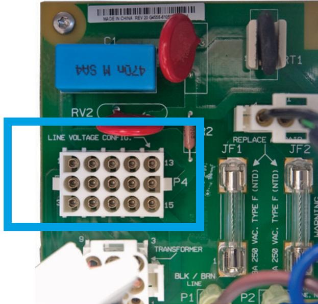
**Figure 1** Close up of AC board
