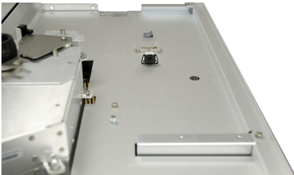
Figure 8 Top base plate installed
