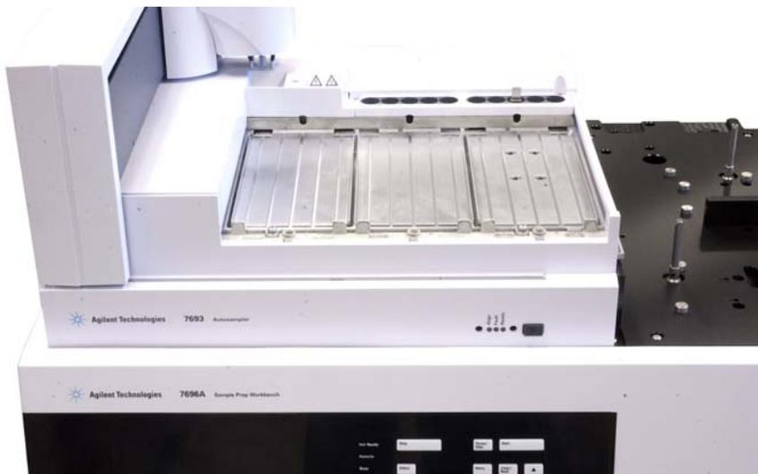
**Figure 55** Sample tray with Peltier module sitting evenly on the main frame surface
