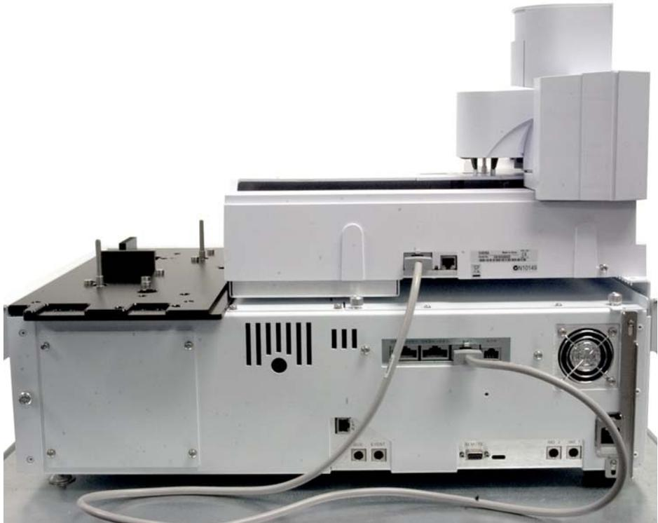
**Figure 15** Connecting the Sample Tray communication cable
