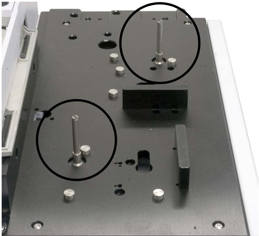
**Figure 18** Installing the mounting posts.
