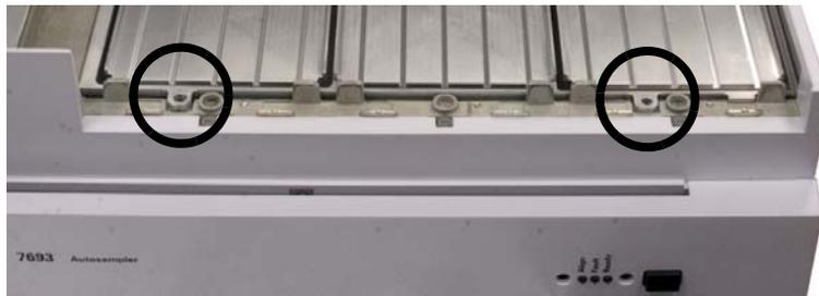
**Figure 48** Installing two T-20 Torx screws to secure the front of the Peltier module
