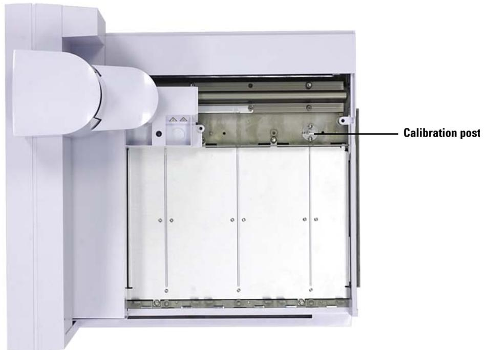
**Figure 40** Removing the unknown vial station
