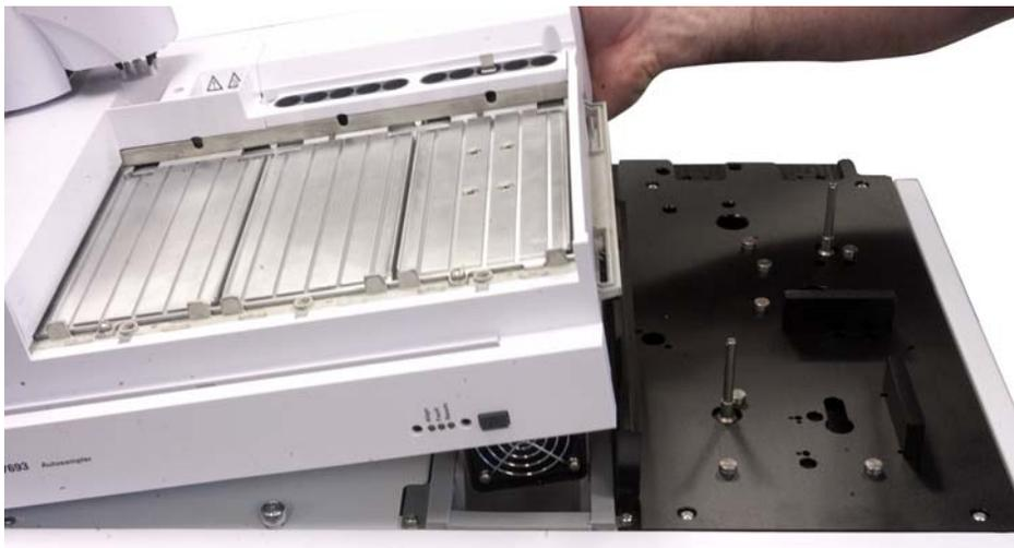
**Figure 54** Lowering the sample tray onto the main frame chassis
