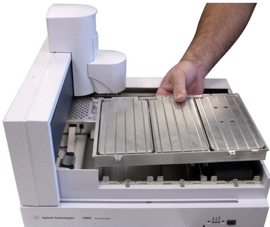
**Figure 46** Installing the Peltier module
