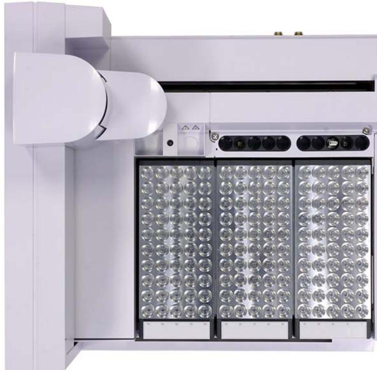
**Figure 58** Installed Peltier module vial racks
