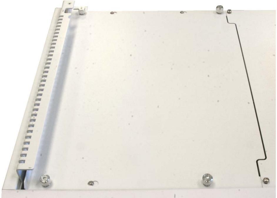
**Figure 27** Removing the top-left main frame cover
