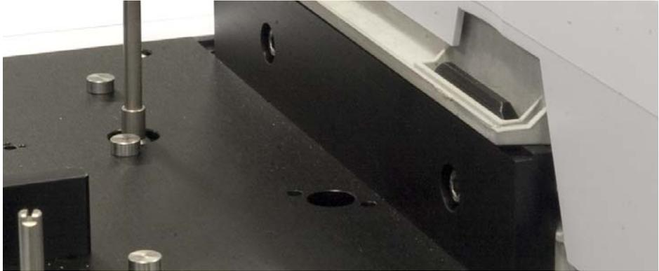
**Figure 26** Removing the screws in the main frame mounting bracket
