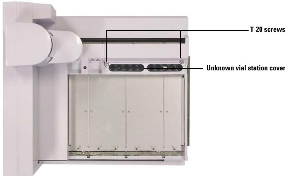
**Figure 39** Removing screws and unknown vial station cover
