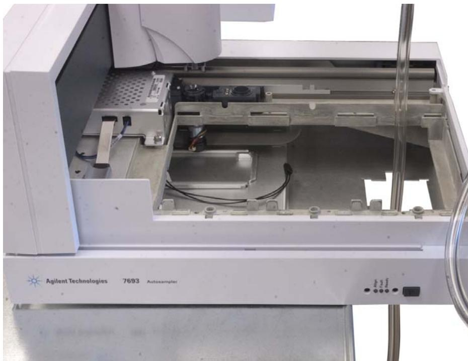
**Figure 44** Running the drainage tubing through the accessory opening
