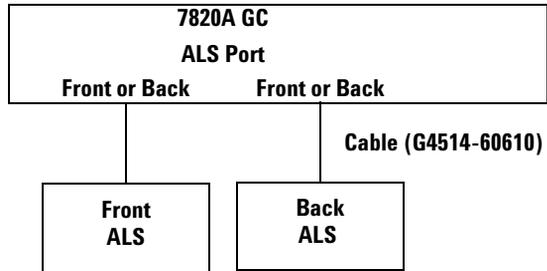
**Figure 21** Cables for 7820A GC
