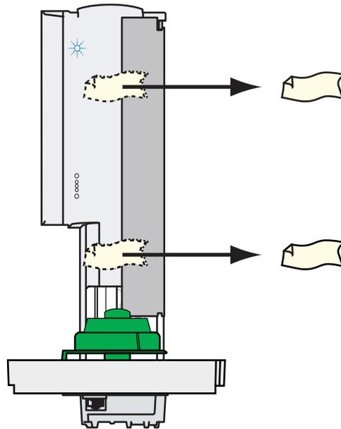
**Figure 5** Remove the shipping tape
