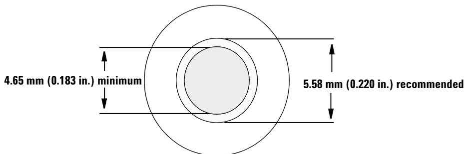
**Figure 37** Vial cap aperture specifications
