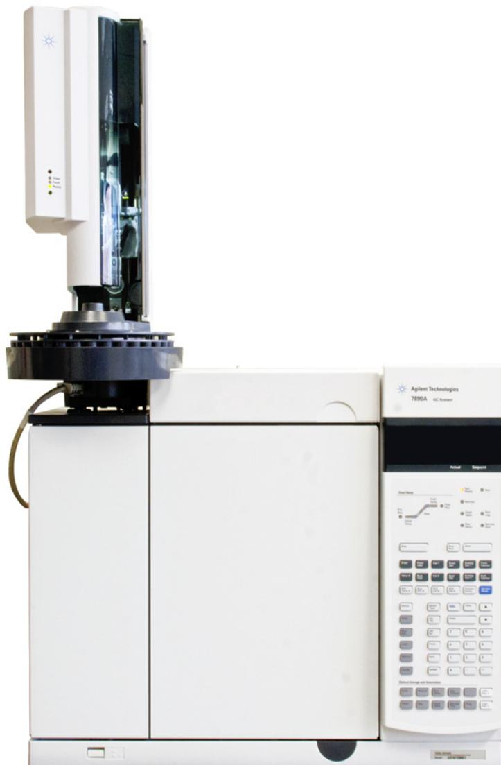
**Figure 18** ALS installed on a 7890A GC
