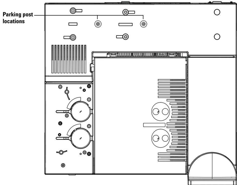
**Figure 72** Parking post positions on a 7890A GC
