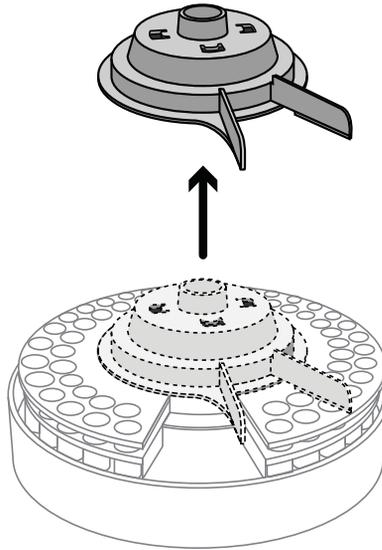
**Figure 56** Removing the turret
