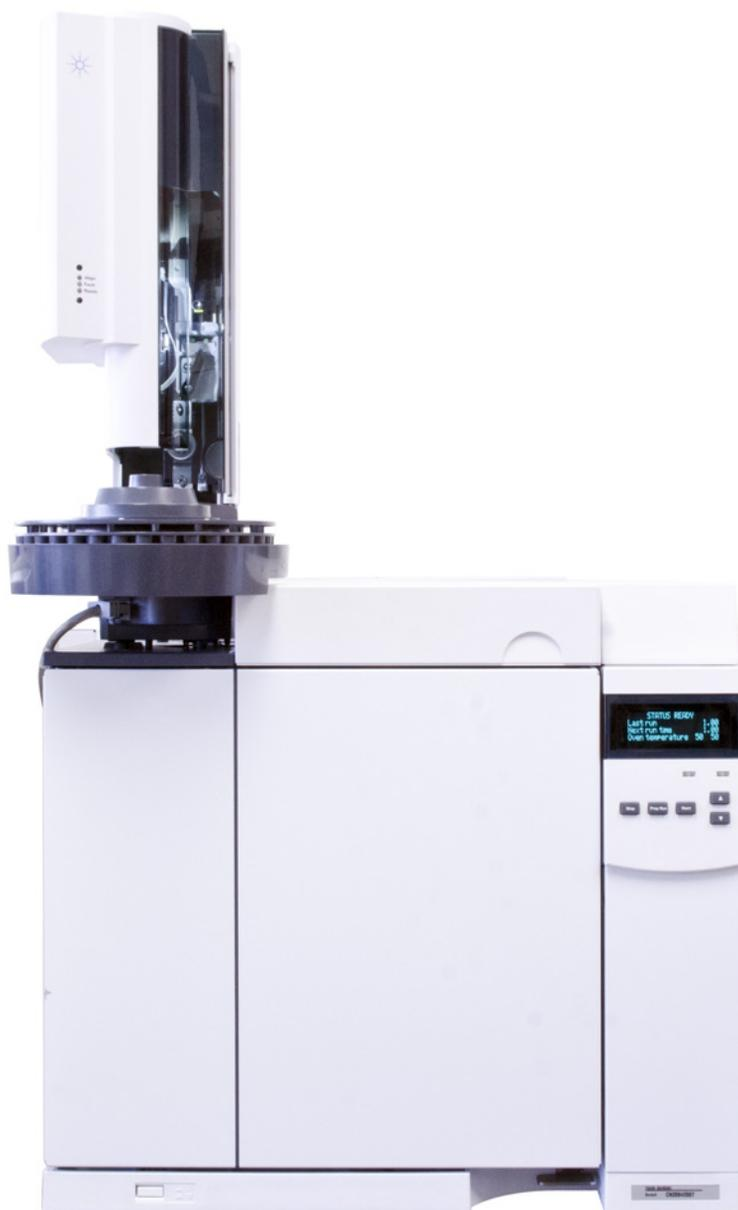
**Figure 19** ALS installed on a 7820A GC
