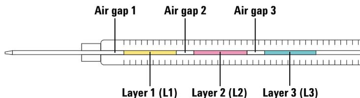
**Figure 47** 3-layer sandwich injection
