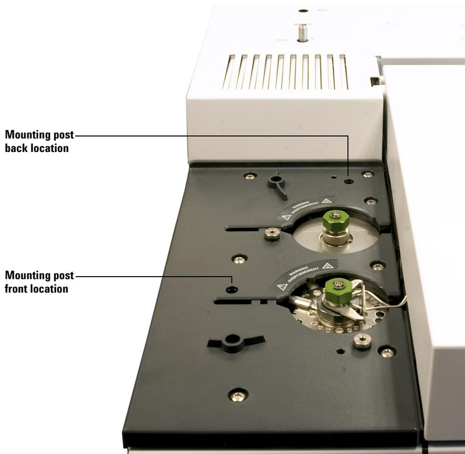
**Figure 14** Mounting post locations on a 7820A GC (7890A GC is similar)
