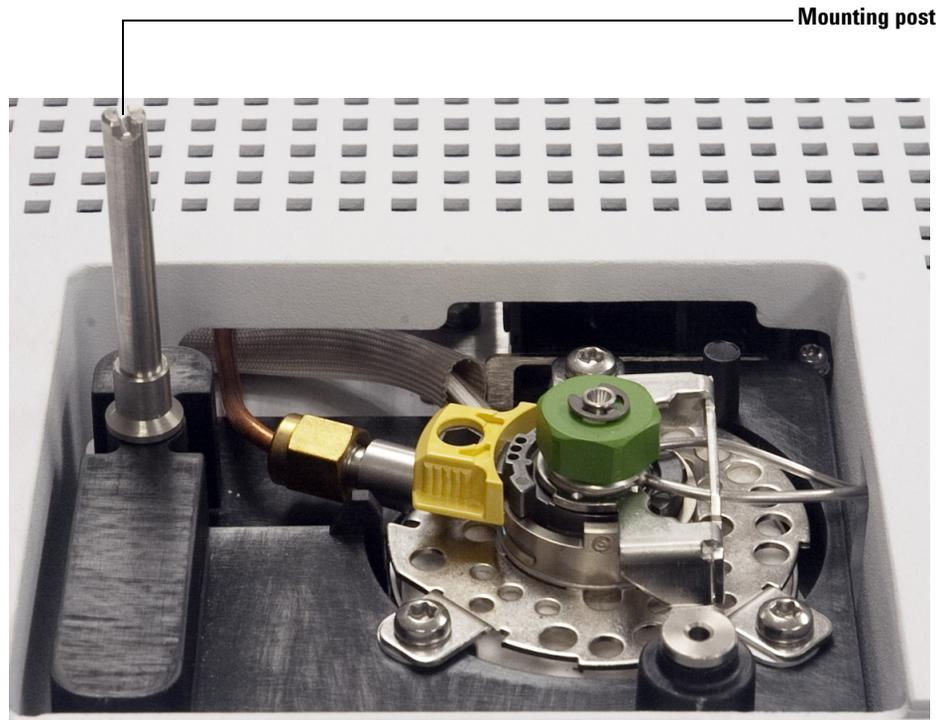
**Figure 15** Mounting post installed on a 5975T LTM-GC/MSD
