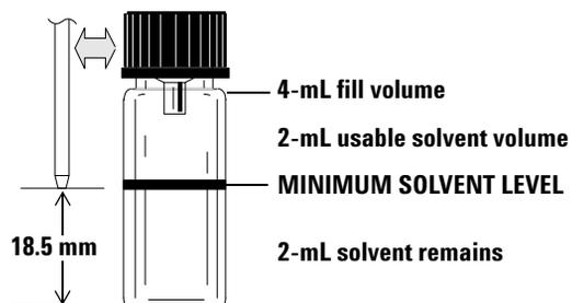
**Figure 43** Needle tip position when withdrawing solvent
