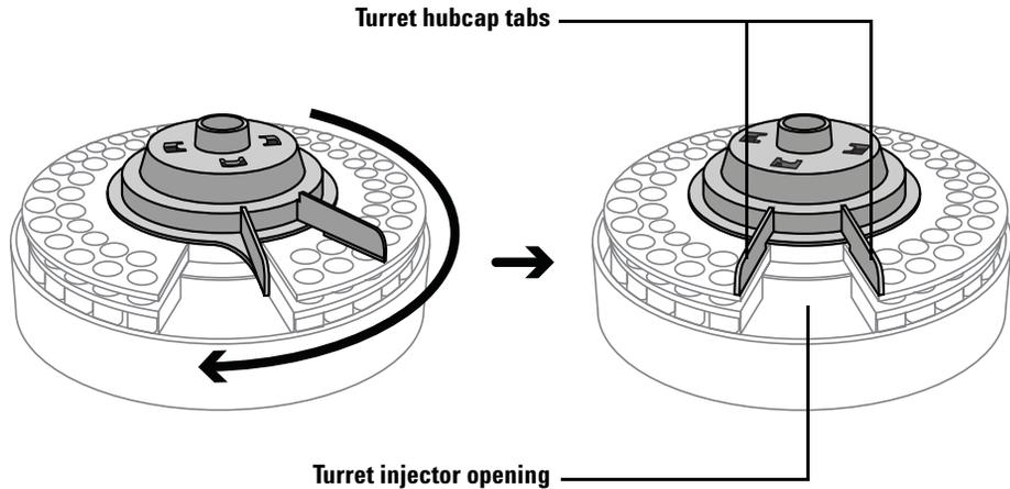
**Figure 62** Rotate the turret hubcap in a clockwise direction until it snaps into position
