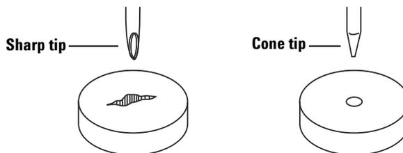
**Figure 29** Needle tips
