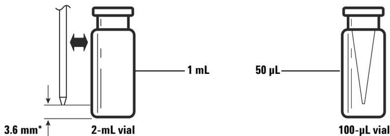
\* Needle position based on default sampling depth
