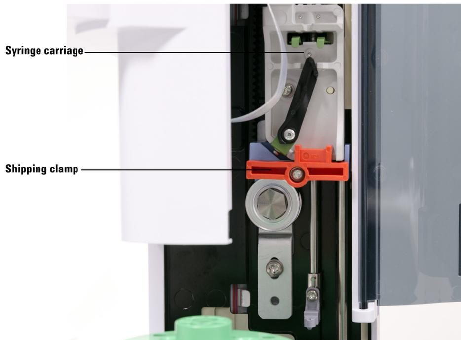
**Figure 4** Shipping clamp installed
