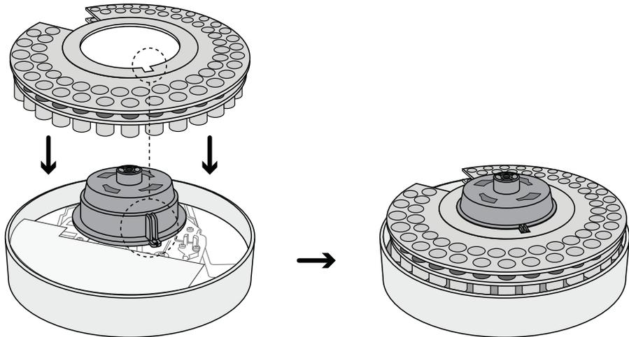
**Figure 9** Place the turret onto the turret hub
