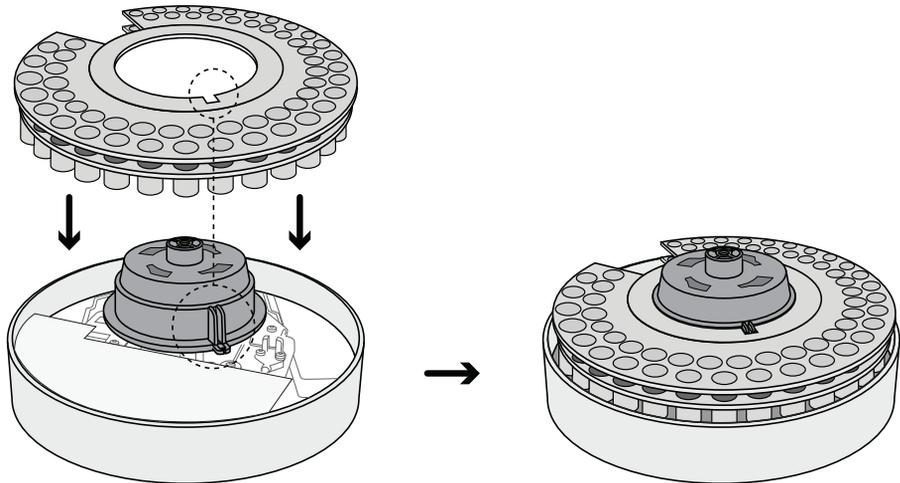
**Figure 59** Place the turret onto the turret hub
