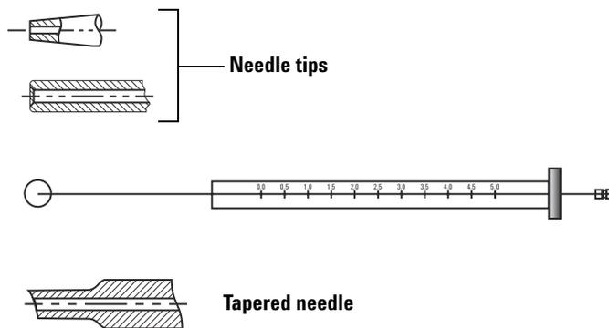
**Figure 30** Needle shapes
