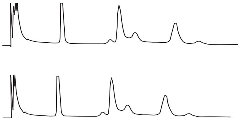
**Figure 73** Retention times or areas are not reproducible
