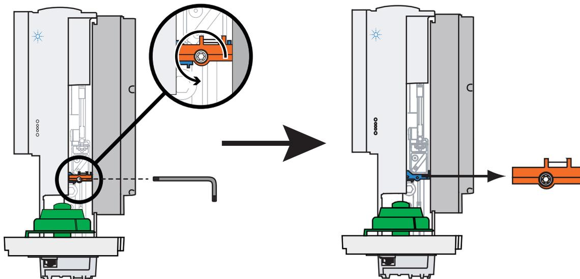
**Figure 6** Remove the orange shipping clamp
