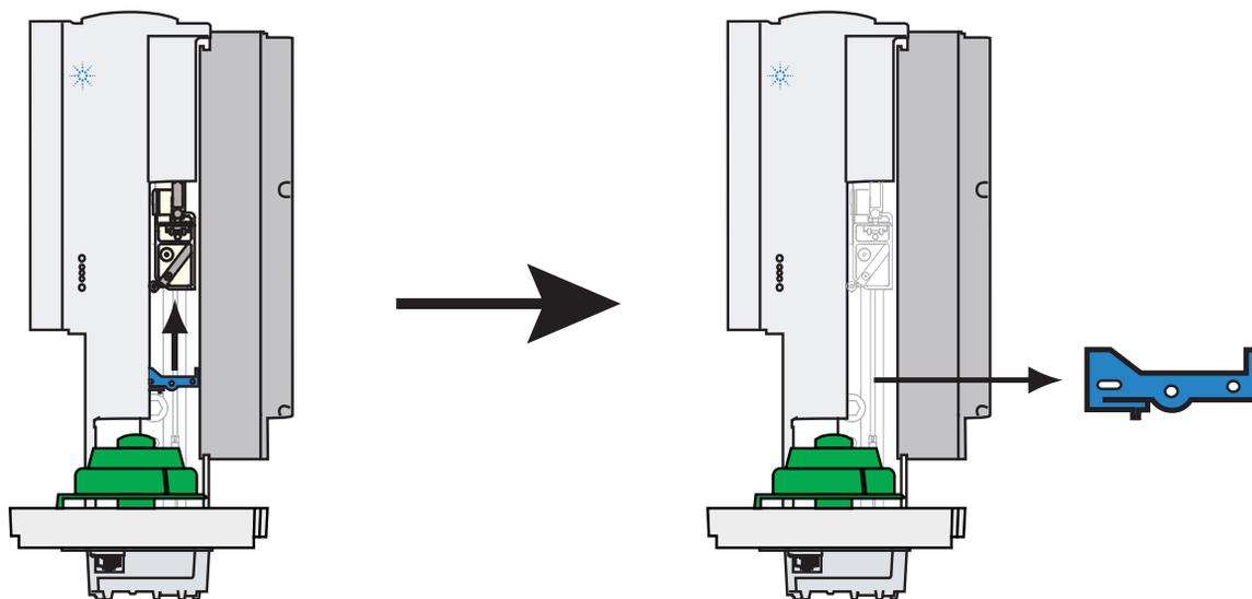
**Figure 7** Remove the blue shipping clamp
