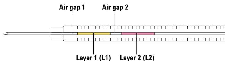
**Figure 46** 2-layer sandwich injection
