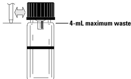
**Figure 44** Needle tip position when discharging waste
