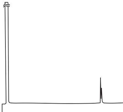
**Figure 75** Blank run showing carryover peaks
