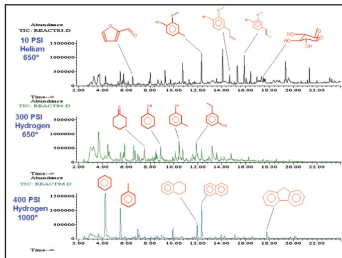
*Wood biomass pyrolyzed at temperature and pressures as noted in either He or H<sub>2</sub>. Runs two and three were passed through a Pt catalyst at 200°C.*
