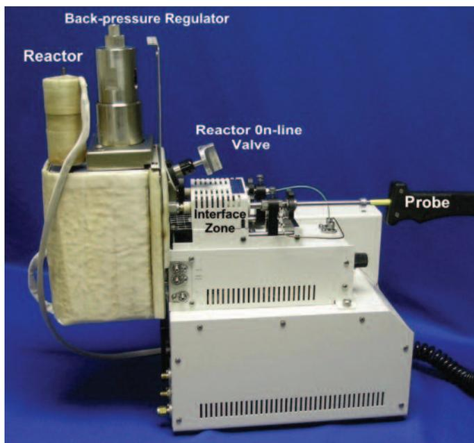
Scientists studying new biomass feedstock, coal, catalysts or chemical reactions need to know how these materials break down in a variety of conditions. Historically this has been a cumbersome, expensive, and time-consuming process. Now there's a better way, the world's first, and only, mini high-pressure pyrolysis reactor system – complete with catalyst reactor.
