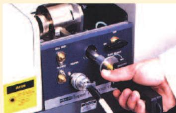
FTIR Interface Mounted in Instrument
