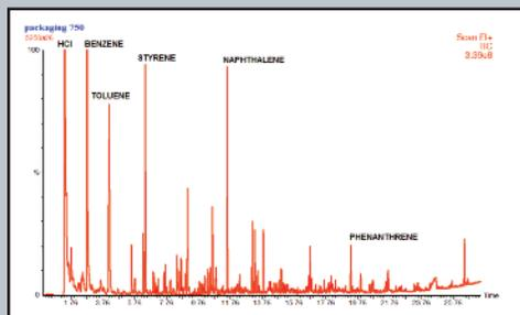
At 750°C the HCl and aromatics identify the polymer as polyvinyl chloride.
