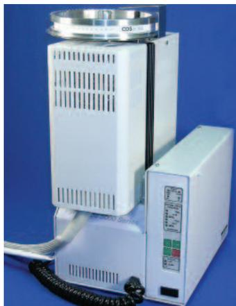
The Model 5250 provides hands-free analysis of up to 36 samples, with the option of expanding to 44. Solids, viscous liquids, and powder samples are pyrolyzed directly into the GC, eliminating the need to perform lengthy extractions and derivatizations.
