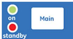
ON: Turns on front panel displays and high voltage to the PMT.
