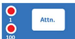
Changes the gain of the amplifier by a factor of 100. For high sensitivity measurement of sulfur or nitrogen compounds (measurement of low levels of sulfur or nitrogen compounds), the attenuation should be operated in the 1 position. For samples containing high levels (ppm to percent) of sulfur or nitrogen compounds, use the 100 position.
