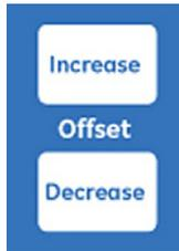
The baseline signal from the SCD and NCD can be adjusted from 0 to  $\pm 1\%$  of the full scale recorder output using the offset control. (e.g., +10 mV to -10 mV for a 1 V full scale setting). This control can be used to offset the background signal.
