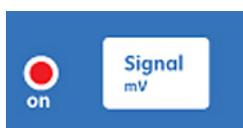
Displays the output signal of the SCD in millivolts. (Note: Changing the output range of the SCD by adjusting the recorder switch on the back panel **does not** change the range of the display.)
