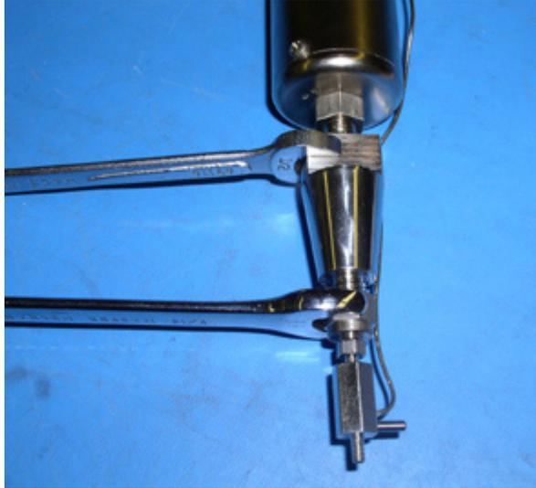
**Figure 30** Tightening the Heater Swivel Nut
