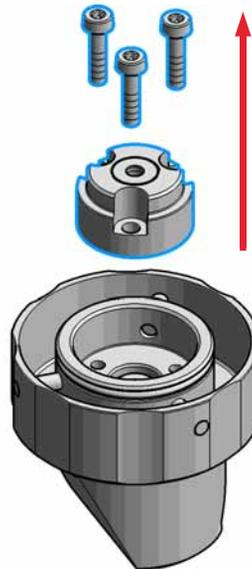
**11** Carefully remove the metering seal using the steel side of the insert tool. Clean the chamber with an appropriate solvent and ensure that all particulate matter is removed.
