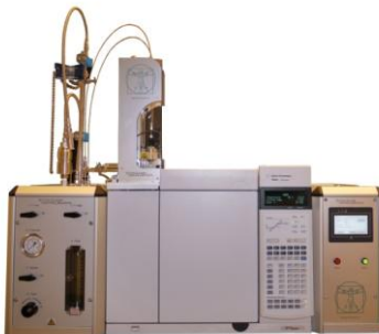
Figure 1: GC System dedicated to the Liquefied Gas Injector
