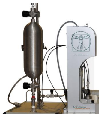
Figure 3: Gasoline Direct Injector transformed into a GC Injector
