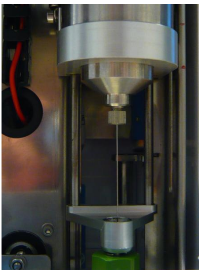
Needle and finger tight needle nut connection
