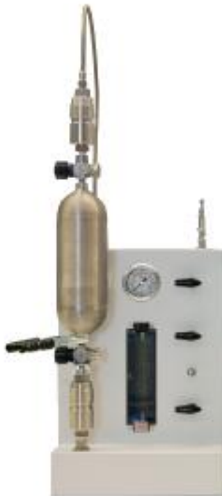
Pressure Station type PTS2 with sample cylinder
