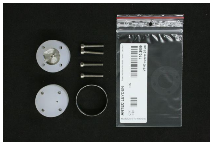
Fig. 13. Disassembled VT-03 micro flow cell with spacer. Note: new VT-03 micro cells purchased after 2009 are delivered without metal centring ring and have no groove in WE and inlet block.
