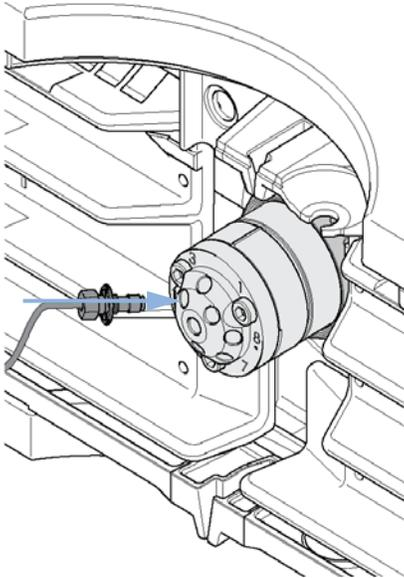
**4** Push the valve head until it snaps in and stays in the rear position. (TCC only)
