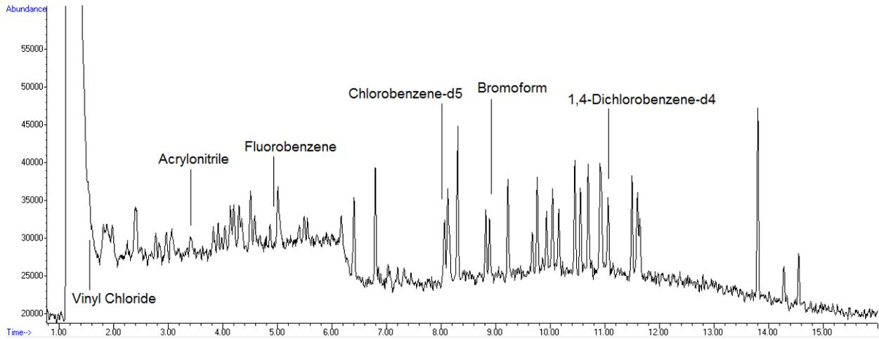
Figure 1: Total Ion Chromatogram of a 5ppb Standard with the Static HT3 Headspace Parameters. The compound retention times are located on the chromatogram.
