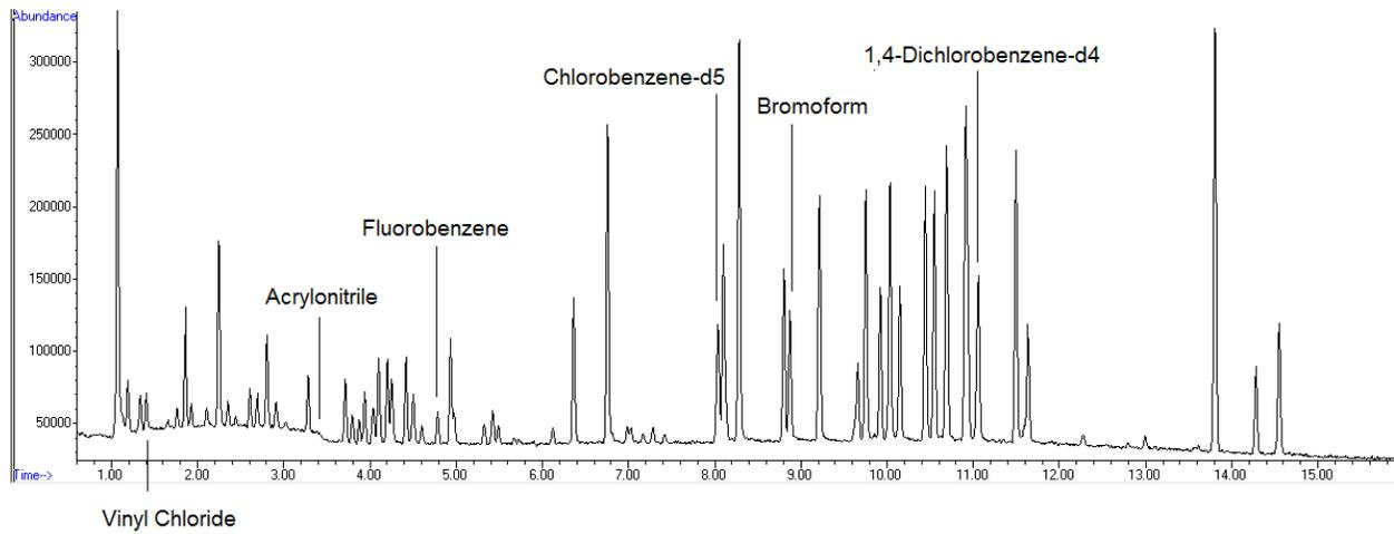
Figure 2: Total Ion Chromatogram of a 5ppb Standard with the Dynamic HT3 Headspace Parameters. The compound retention times are located on the chromatogram.
