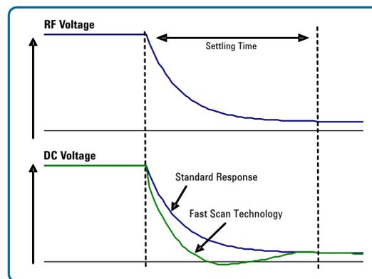
Figure 2: Standard and Fast Scan Response Curves
