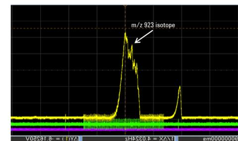
Figure 3: Oscilloscope trace of m/z 922 collected from detector amplifier while scanning at 10 KDa/sec
