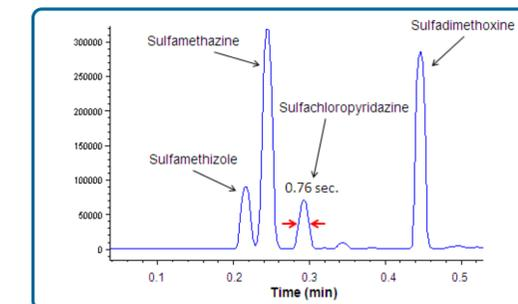
Figure 5: UHPLC chromatographic data at 15 KDa/sec
