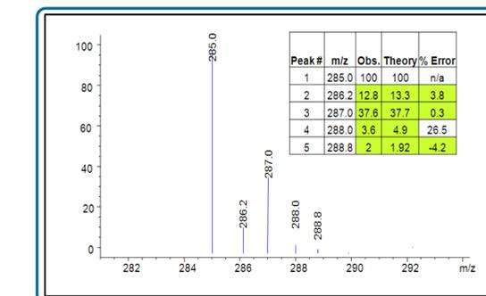
Figure 6: Mass spectrum and isotope distribution of sulfachloropyridazine collected at 15 KDa/sec.
