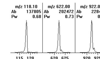
Figure 4b: Linear Phase FIR filtering at 15 KDa/sec
