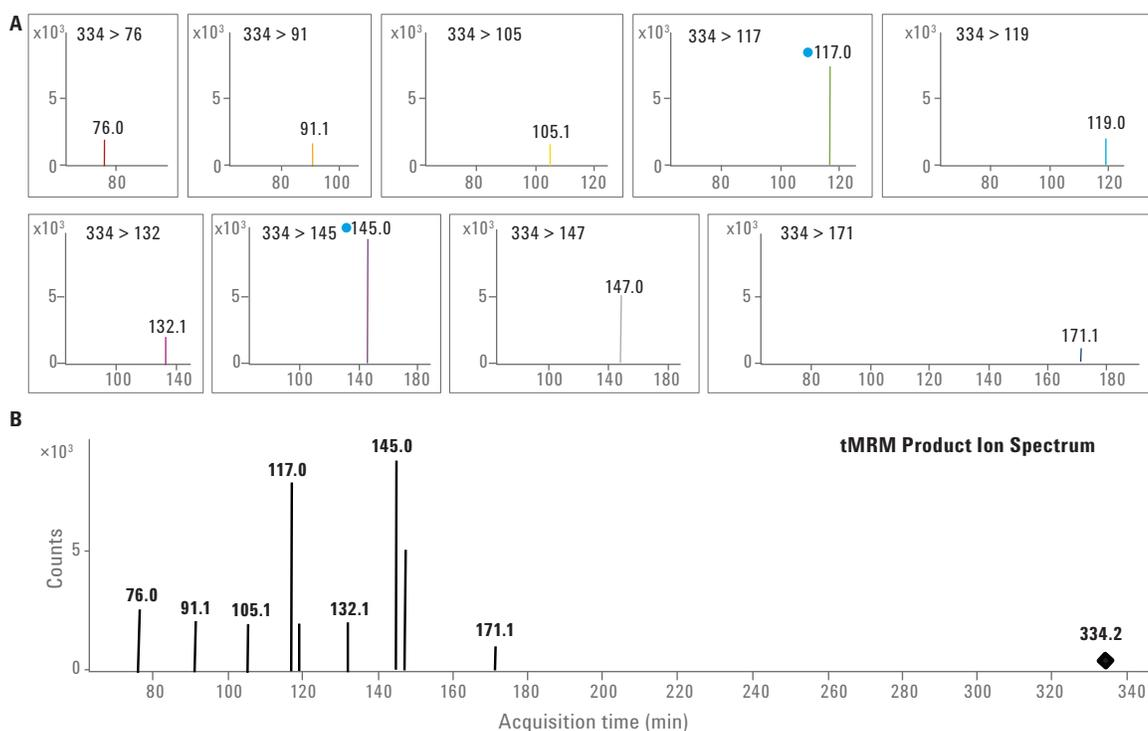
Figure 2. tMRM product ion spectra are generated by combining the primary (●) and secondary MRM spectra for a target analyte **A**. The product ion spectrum **B** may be used for library search and analyte confirmation.
