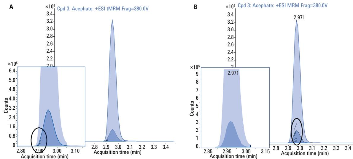
Figure 3. Data acquired for acephate using the entrance delay triggering function.
